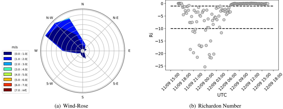
Figure 2: Flow conditions during PIV experiments. In subfigure (b), the dashed lines represents the boundaries of forced ( $Ri = -1$ ) and natural convection ( $Ri = -10$ ). In between, the flow regime is mixed convection.
