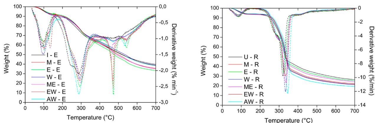
**Figure 2.** Thermograms of the chestnut wood extracts (left) and residues (right) at  $10\text{ }^{\circ}\text{C min}^{-1}$  under nitrogen flow as a function of solvent nature compared to the industrial extract (I-E) and the untreated chestnut wood (U-R).
