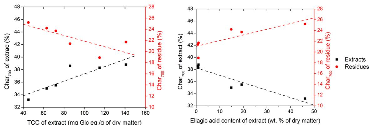
**Figure 3.** (A) Char yield at 700 °C of the chestnut wood extracts and residues versus total carbohydrate content (TCC) in the associated chestnut wood extracts. (B) Char yield at 700 °C of the chestnut wood extracts and residues versus ellagic acid content in the associated chestnut wood extracts. The standard deviations of triplicate assays are available in the [Supporting Information](#).
