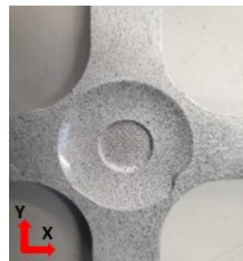
Figure 5. Painted specimen for the DIC
