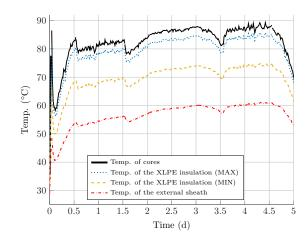
Fig. 7. Temperature calculated in different locations of the cable for Case 3, i.e. with a wave farm composed of 12 to 15 WECs. As we can see, the cable cores temperature is very close to  $T_{max} = 90$  °C.
