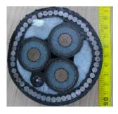
Fig. 3. Cross section picture of the export cable considered for our case studies. This  $3 \times 95 \text{ mm}^2$  copper cores cable (that was designed to carry a constant electric current of 290 A) is currently installed in the SEM-REV test site located off Le Croisic (see Fig. 2), France and is managed by École Centrale de Nantes [16].
