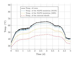
Fig. 5. Temperature calculated in different locations of the cable for Case 1, i.e. with a wave farm composed of 11 WECs. As we can see, the cable cores temperature are far from  $T_{max} = 90$  °C, as allowed by the manufacturer and suggested in IEC standards.
