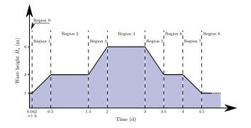
Fig. 4. Sequence of sea-states that has been used for all simulation cases (see Table I). Note that it is a completely fictitious sequence but based on plausible durations and transitions between each sea-states based on Fig. E2 and E3 of [17].
