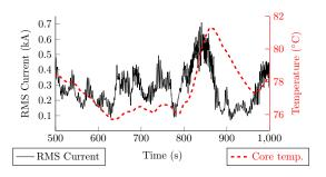
Fig. 1. Example of a RMS current profile generated by a WEC farm composed of 20 WECs considering a  $H_s = 6$  m and  $T_p = 9$  s sea-state. The current profile is very fluctuating and ranges between 70 A and 700 A while in the same time the temperature varies only from 76°C to 81°C.
