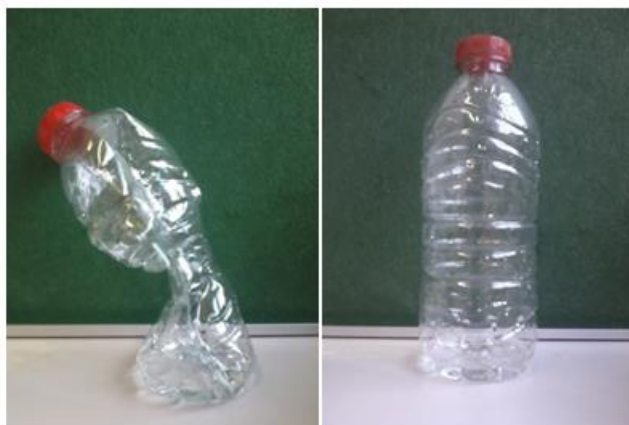
305 Figure 5. Plastic bottles filled with sodium hydroxide solution and \text{CO}_2 (left), and filled with sodium hydroxide solution and air (right). The NaOH solution absorbs \text{CO}_2 but not air, hence only the bottle that contains \text{CO}_2 has contracted. This interactive demonstration helped support the explanation that liquid solvents could absorb gaseous \text{CO}_2 .
