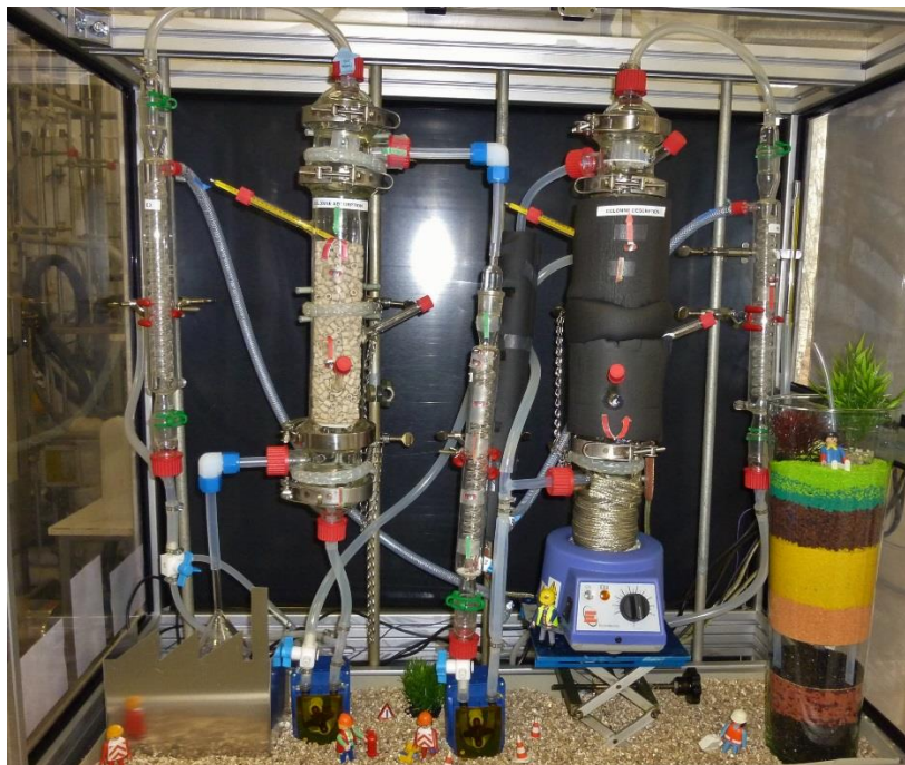
Figure 1. Carbon dioxide capture pilot plant designed and manufactured by the student project team.
