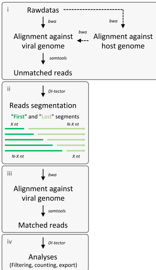
FIGURE 2. Schematic representation of the DI-tector workflow, which includes four main steps: (i) alignment against host and viral genomes to collect unmatched reads, (ii) segmentation, (iii) second alignment against viral genomes, and (iv) analyses of the matched segmented reads. Dashed lines represent optional steps.
