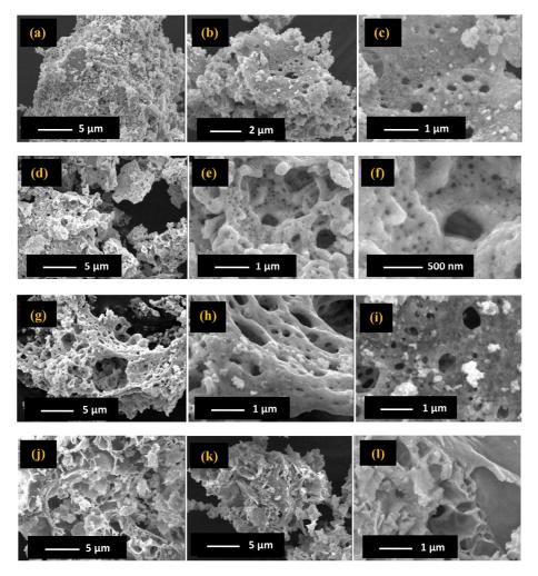
Fig.4. SEM images at different magnification of all catalysts (a-c) CuO-CeO<sub>2</sub>, (d-f) ZnO-CeO<sub>2</sub> (g-i) CuO-ZnO-CeO<sub>2</sub> and (j-l) CuO-ZnO-Al<sub>2</sub>O<sub>3</sub>
