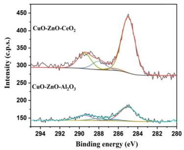
Fig.6. C 1s XPS spectra of CuO-ZnO-CeO<sub>2</sub> and CuO-ZnO-Al<sub>2</sub>O<sub>3</sub> samples
