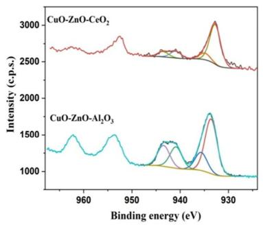
Fig.5. Cu 2p XPS spectra of CuO-ZnO-CeO<sub>2</sub> and CuO-ZnO-Al<sub>2</sub>O<sub>3</sub> samples
