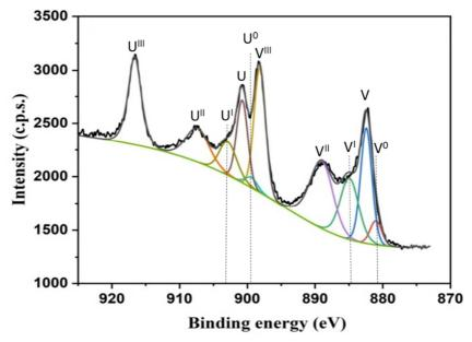
Fig.8. Ce 3d XPS spectra of the CuO-ZnO-CeO<sub>2</sub> sample Spectres XPS Ce 3d de l'échantillon CuO-ZnO-CeO<sub>2</sub>
