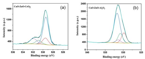
Fig.7. O 1s XPS spectra of (a) CuO-ZnO-CeO<sub>2</sub> and (b) CuO-ZnO-Al<sub>2</sub>O<sub>3</sub> samples
