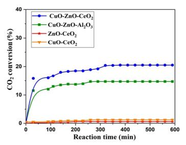
**Fig.9.**  $CO_2$  conversion as function of the time of reaction. Reaction conditions:  $CO_2/H_2 = 1/9$ ,  $T=240^{\circ}C$ , flow=1L.h<sup>-1</sup> and P=1 atm.
