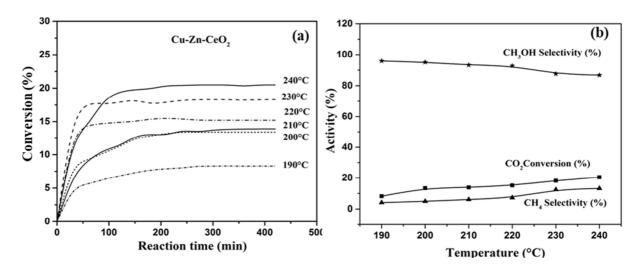
**Fig.10.** a)  $CO_2$  conversion as function of the time and temperature of reaction b)-MeOH and  $CH_4$  selectivity as function of the temperature of reaction, over the CuO-ZnO- $CeO_2$  catalyst:  $flow=1L.h^{-1}$  and P=1 atm
