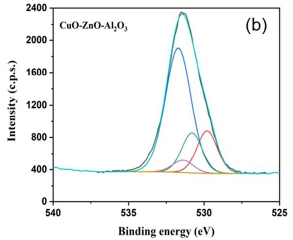
**Fig.7.** O 1s XPS spectra of (a) CuO-ZnO-CeO<sub>2</sub> and (b) CuO-ZnO-Al<sub>2</sub>O<sub>3</sub> samples
