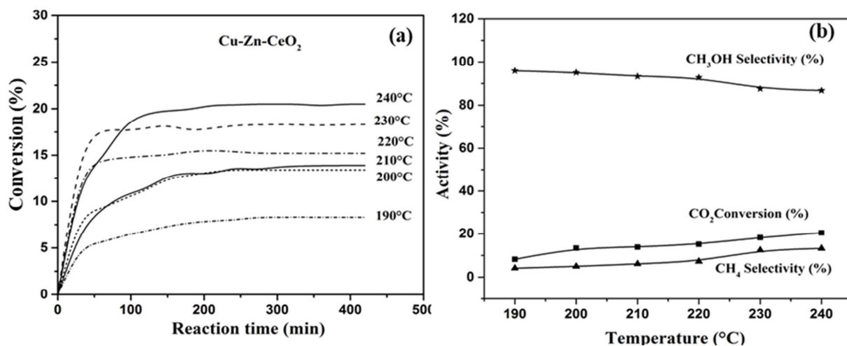
**Fig.10.** a) CO<sub>2</sub> conversion as function of the time and temperature of reaction b)-MeOH and CH<sub>4</sub> selectivity as function of the temperature of reaction, over the CuO-ZnO-CeO<sub>2</sub> catalyst: flow=1L.h<sup>-1</sup> and P = 1 atm
