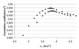
Fig. 4. Correlation coefficient  $r^2$  as a function of applied threshold velocity  $(u_i; \text{m s}^{-1})$  for the regression lines comparing the total sand fluxes from all BSNE locations for each of the eight sandstorms using the QUIC wind velocities at heights 0.625 m for the White (gray squares) and Owen (black triangles) equations and the field measurements. The optimal  $u_t$  value at 0.625 m is 5.8 m s<sup>-1</sup>, for both Eqs. (1) and (2).
