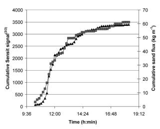
Fig. 10. Cumulative Sensit counts to the 3/2 power (solid triangles) as a function of time, plotted with predicted cumulative sand flux (kg m<sup>-1</sup>) from the White equation (solid squares) at the Sensit location for the largest storm on 15 Apr 2003.
