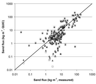
Fig. 7. Total sand flux (kg m<sup>-1</sup>) predicted by QUIC for each storm for each BSNE collector as a function of the measured sand flux. Solid triangles and open squares show the approximations based on the 0.625-m velocity predictions for the Owen and White equations, respectively.
