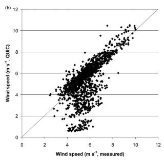
Fig. 2. (a) Wind velocity vectors (0.625-m height) at the study site (bushes and dunes are black) are shown for one 10-min time period on 15 Apr 2003. The reference wind velocity at 14.9 m was 15.3 m s $^{-1}$  at 234°. (b) The comparison for six locations between all of the 10-min-averaged wind speeds measured in the field (scaled to a 0.625-m height) and the predictions made by QUIC.
