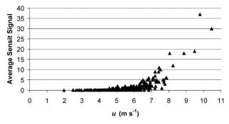
Fig. 6. The 10-min average of Sensit counts vs wind velocity measured at 0.75 m on mast N during the 2003 experiment.
