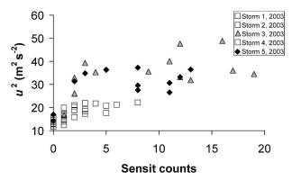
Fig. 12. The square of the wind speed predicted by QUIC at the Sensit location as a function of measured Sensit counts (for the wind direction measured at the 15-m tower between 220° and 239°).
