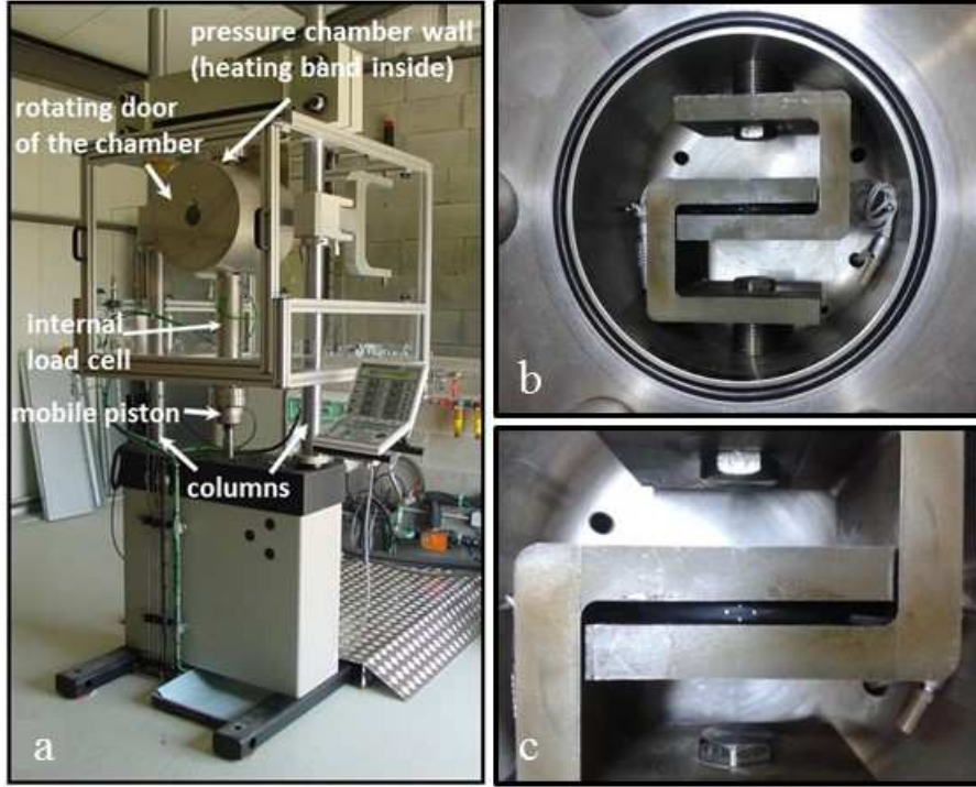
Figure 1. a) global view and (b) magnification of the pressure CO 2 chamber of the experimental testing machine. (c) Specific U-shaped mounting for seal compression
