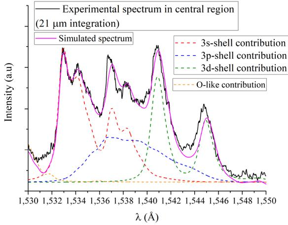
Figure 6: Spatially integrated spectrum observed in the central part of the plume between 42 and 63  $\mu\text{m}$ . The pink curve shows the best fit. The other curves show the contribution from each subshell. The O-like contribution at the very left-hand part of the spectrum is also included.
