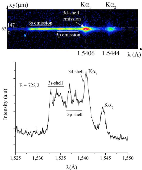
Figure 2: Spectrum recorded with the FSSR-1D and the reconstructed integrated profile. The emission of all M-shell charge states is divided in three sub-structures, 3d, 3p and 3s.
