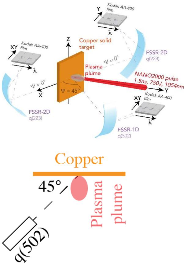
Figure 1: a. Scheme of the experimental setup includes two FSSR-2D spectrometers covering a large bandwidth from  $K\alpha$  to  $Ly\alpha$  lines and one FSSR-1D with a narrow bandwidth centered on M-shell copper charge states. b. Scheme of the setup from the top showing the main diagnostic angle of view.
