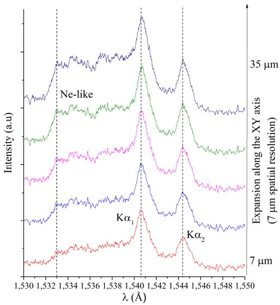
Figure 4: *a.* Spatially resolved spectrum recorded using FSSR-1D in steps of 21 μm. Between -42 and 0 μm (along the target), only the emission of 3d-shell states is visible. Emission from the plasma plume shows higher ionization states and variations in ionic fractions. Dashed lines represent the position of the cold Kα lines that shift to the red in the hot material.
