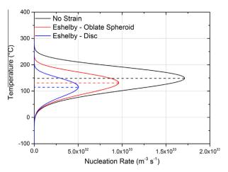
Fig. 7. Calculated nucleation rate as a function of temperature, strain energy and geometry.
