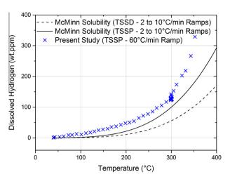
Fig. 5. Predicted and recorded hydrogen in solution curves [60].
