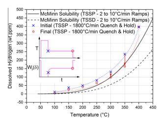
**Fig. 6.** Supersaturation in isothermal holds after quenching from rate limited kinetics [60].
