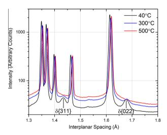
**Fig. 2.** Representative diffractograms from 40 °C, 300 °C and 500 °C acquisitions for the considered range of lattice spacing.
