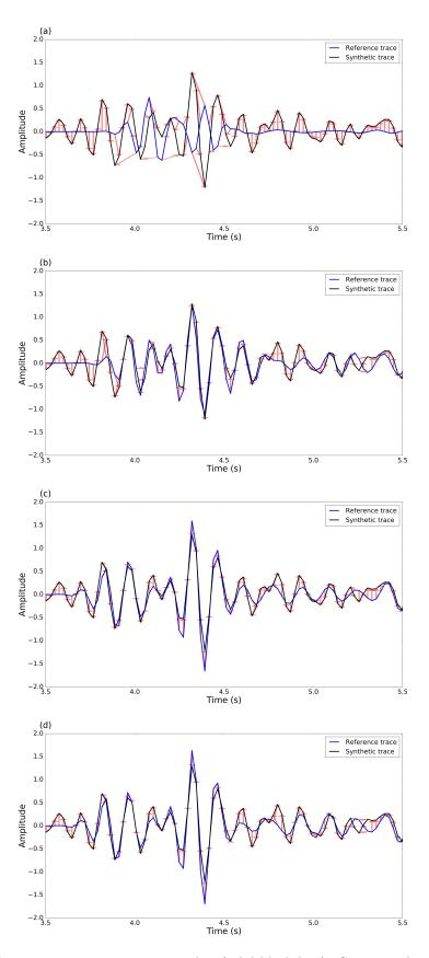
Figure 19: Reference seismic trace at  $x_r = 7$  km (solid black line). Corresponding synthetic trace (solid blue line) in the initial model (a), 10th iteration model (b), 50th iteration model (c), final model (d). The assignment solution of the graph space OT problem between the synthetic and reference trace is presented in orange arrows.
