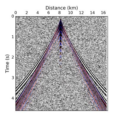
Figure 4: Observed data in the reference model with  $\gamma = 0.7$  and  $v_{P,0} = 2000 \text{ m.s}^{-1}$  (black and white). Synthetic data in the model with  $\gamma = 0.45$  and  $v_{P,0} = 1750 \text{ m.s}^{-1}$  (blue and red). We measure a maximum time shift at the largest offset equal to 0.46 s.
