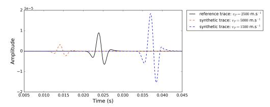
Figure 6: Signal recorded for the three considered homogeneous media: reference medium at  $2500 \text{ m.s}^{-1}$  (solid black line), slower medium at  $1500 \text{ m.s}^{-1}$  (dashed blue line), faster medium at  $5000 \text{ m.s}^{-1}$  (dashed orange line).
