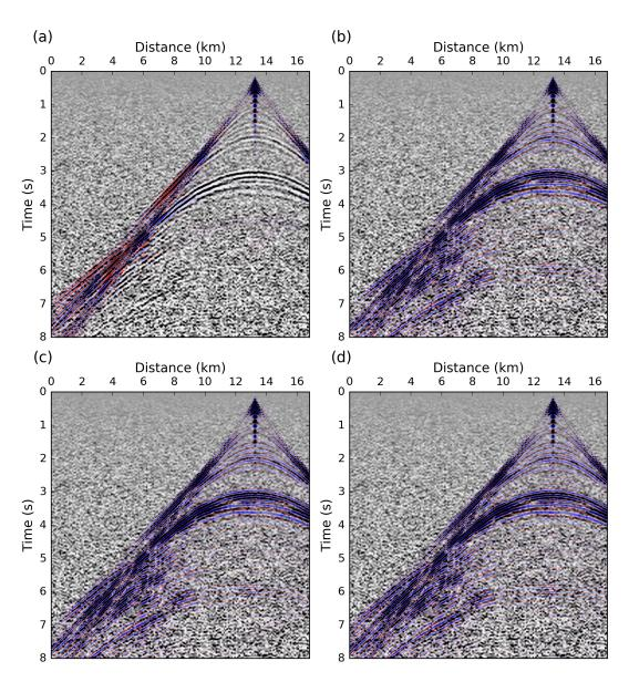
Figure 13: Data fit in the initial model 1 (a), and in the reconstructed model from model 1 using the  $L^2$  misfit function (b), the KR misfit function (c), the graph space OT misfit function (d). The real data is represented in black and white, while the synthetic data computed in the corresponding models is represented in red and blue. When the synthetic data predicts correctly the true data, the blue overlays the white events, while the black overlays the red events.
