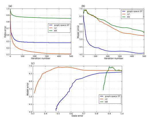
Figure 18: Convergence analysis for the inversion starting from the initial model 3. Misfit function decrease depending on the number of iterations (a). Model error depending on the number of iterations (b). Model error depending on the data error (c).
