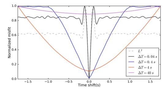
Figure 3: Comparison of the graph-space OT misfit function depending on the time shift, for different values of the parameter  $\Delta T$ . The reference least-squares misfit is in dashed gray line. Solid black line: misfit function for  $\Delta T = 0.04$  s. Solid blue line: misfit function for  $\Delta T = 0.4$  s. Solid orange line: misfit function for  $\Delta T = 4$  s. Solid purple line: misfit function for  $\Delta T = 40$  s.
