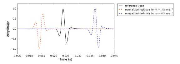
Figure 7: Reference signal for the medium at  $2500 \text{ m.s}^{-1}$  (solid black line). Corresponding graph space OT adjoint source for the slower medium at  $1500 \text{ m.s}^{-1}$  (dashed blue line), faster medium at  $5000 \text{ m.s}^{-1}$  (dashed orange line).
