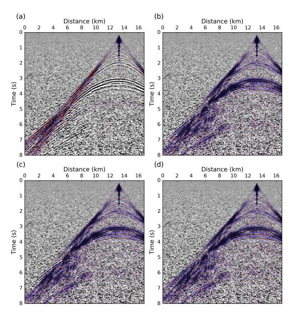
Figure 17: Data fit in the initial model 3 (a), and in the reconstructed model from model 3 using the  $L^2$  misfit function (b), the KR misfit function (c), the graph space OT misfit function (d). The real data is represented in black and white, while the synthetic data computed in the corresponding models is represented in red and blue. When the synthetic data predicts correctly the true data, the blue overlays the white events, while the black overlays the red events.
