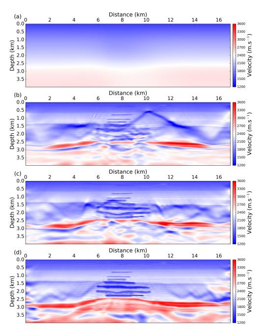
Figure 20: Initial model 4 (a). Corresponding reconstructed models using the  $L^2$  misfit function (b), the KR misfit function (c), the graph space OT misfit function with a hierarchical approach using decreasing values of  $\Delta T$ : 0.5 s, 0.4 s, 0.2 s, 0.8 s, 0.4 s and 0.2 s.
