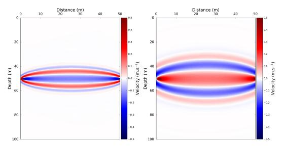
Figure 8: Gradient of the graph-space OT misfit function computed in the slower medium  $1500 \text{ m.s}^{-1}$  (left) and in the faster medium at  $5000 \text{ m.s}^{-1}$  (right).
