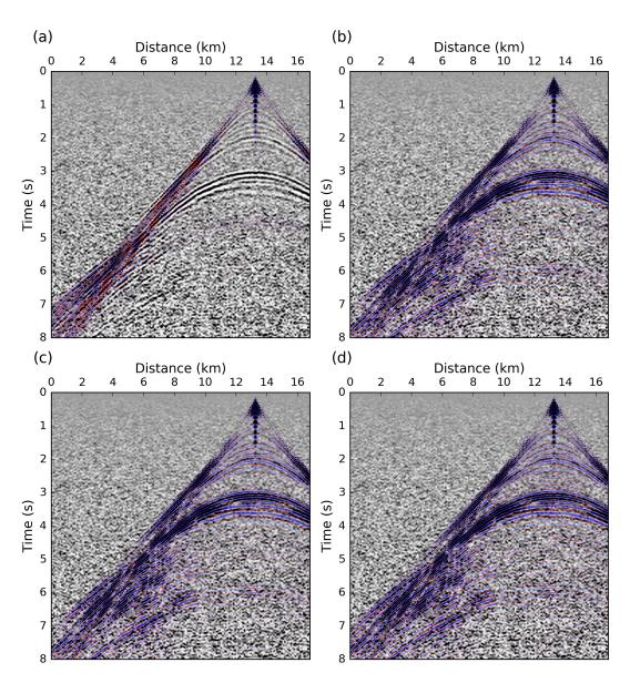
Figure 15: Data fit in the initial model 2 (a), and in the reconstructed model from model 2 using the  $L^2$  misfit function (b), the KR misfit function (c), the graph space OT misfit function (d). The real data is represented in black and white, while the synthetic data computed in the corresponding models is represented in red and blue. When the synthetic data predicts correctly the true data, the blue overlays the white events, while the black overlays the red events.
