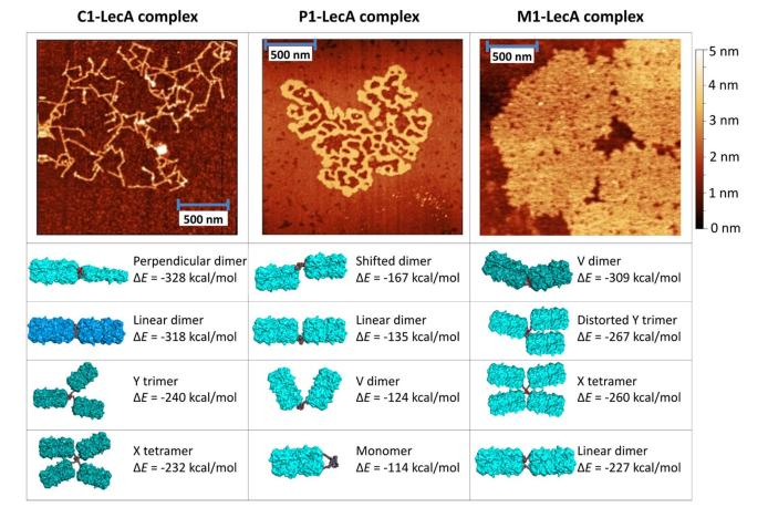
Figure2: AFM topographic images and MD simulations of C1-LecA, P1-LecA and M1-LecA complexes. Image size: 2 x 2  $\mu$ m<sup>2</sup>.
