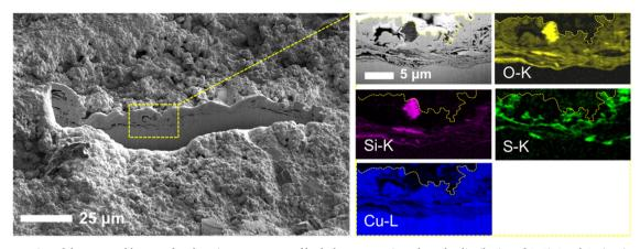
Fig. 9. FIB cross-section of the uncoated bronze after dropping. X-ray maps of both the cross-sections show the distribution of O, Si, S and Cu (Mn is not reported as the EDS map is not well-resolved). Pt-C layer was applied before FIB milling in order to protect the top surface of the cross-section. (For interpretation of the references to colour in this figure legend, the reader is referred to the web version of this article).
