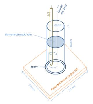
Fig. 1. Electrochemical cell for the preliminary assessment of coating protectiveness.
