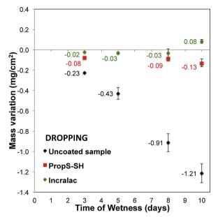
**Fig. 6.** Mass variation for the uncoated (black dataset) and coated bronze samples (PropS-SH and Incralac\* by spraying in red and in green, respectively) during accelerated ageing by dropping test (For interpretation of the references to colour in this figure legend, the reader is referred to the web version of this article).
