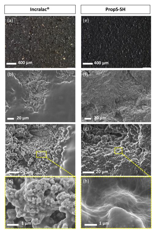
Fig. 4. (a–d) Incralac<sup>\*</sup> and (e–h) PropS-SH surfaces on K<sub>2</sub>S-patinated bronze (spraying application of both the coatings), at different magnifications. Optical and SEM observation (SEI).
