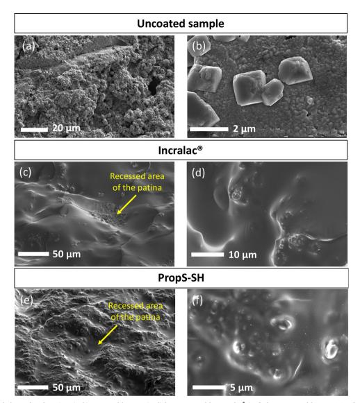
Fig. 8. Surface morphology after dropping: (a, b) Uncoated bronze; (c, d) bronze coated by Incralac\* (e, f); bronze coated by PropS-SH (both the coatings were applied by spraying).
