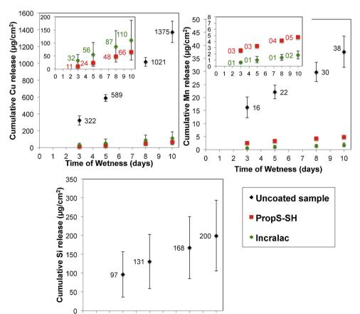
Fig. 7. Cumulative Cu, Mn and Si ions release ( $\mu$ g/cm²) from bronze samples (uncoated and coated by spraying) in acid rain solution, as a function of exposure time, for a total Time of Wetness (ToW) of 10 days of dropping test. Concentration of Si specie is not reported for coated samples, as it is under the Limit of Detection (LoD < 18 ppb). (For interpretation of the references to colour in this figure legend, the reader is referred to the web version of this article).
