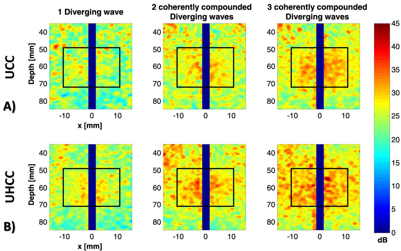
**Figure 7.** SNR maps of Pork-belly-gelatin-agar phantom configuration for UCC (A) and UHCC (B) imaging. The blue boxes represent the push region and the black rectangles represent the SNR regions-of-interest.
