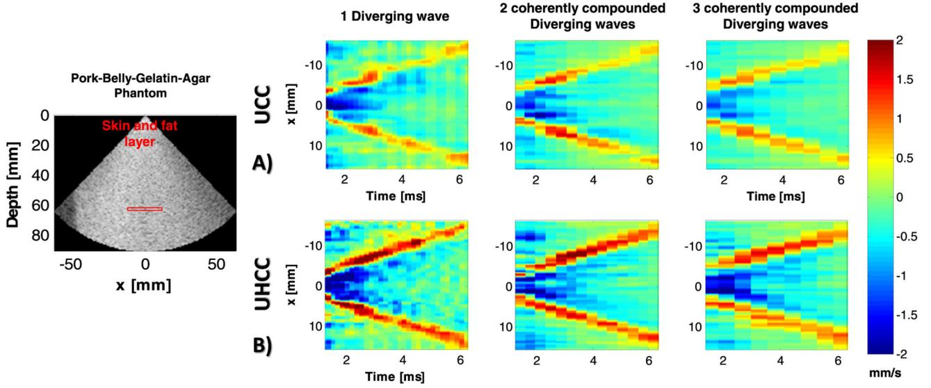
**Figure 5.** Pork-belly-gelatin-agar phantom configuration results. A B-mode ultrafast harmonic using 10 diverging-waves and spatiotemporal tissue velocity images of the shear wave propagation (push-depth 65-mm) for UCC (A) and UHCC (B). SWE using 1, 2, and 3 coherently compounded diverging waves. Tissue velocities were averaged axially within a 3-mm region.
