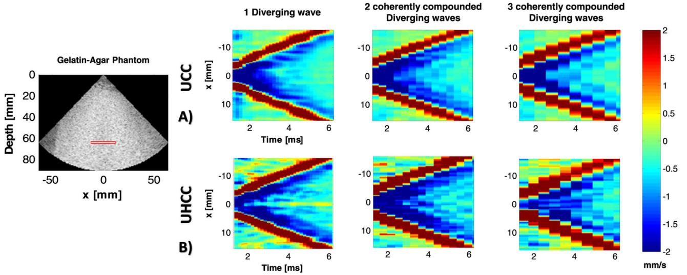
**Figure 4.** Gelatin-agar phantom configuration results. A UHCC B-mode image using 10 diverging-waves and B spatiotemporal tissue velocity images of the shear wave propagation (push-depth equal to 65 mm) for UHCC (B) and UCC (A) SWE using 1, 2, and 3 coherently compounded diverging waves. Tissue velocities were averaged axially within a 3-mm region.
