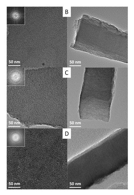
**Figure 2.** TEM micrographs (top views on the left and cross-sections on the right) of mesoporous silica films prepared by EASA from a starting sol containing TEOS and CTAB in the presence of increasing concentrations of Fe(Htrz)<sub>3</sub> complex: 0.5 mM (A), 1 mM (B), 3 mM (C) and 5 mM (D). Electron diffraction patterns are also shown on top view micrographs.
