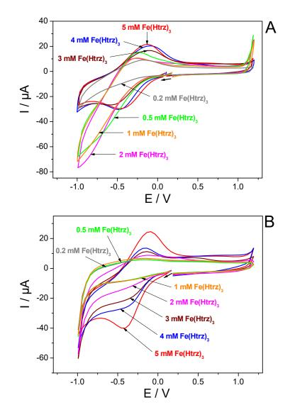
**Figure 1.** Cyclic voltammograms recorded at 0.5 V s<sup>-1</sup> in 0.1 M NaNO<sub>3</sub> aqueous solution using mesoporous silica film modified ITO electrodes prepared from a starting sol containing increasing concentrations of  $Fe(Htrz)_3$  complex (from 0.2 to 5 mM), respectively before (A) and after film treatment in 0.1 M HCl in ethanol (B).
