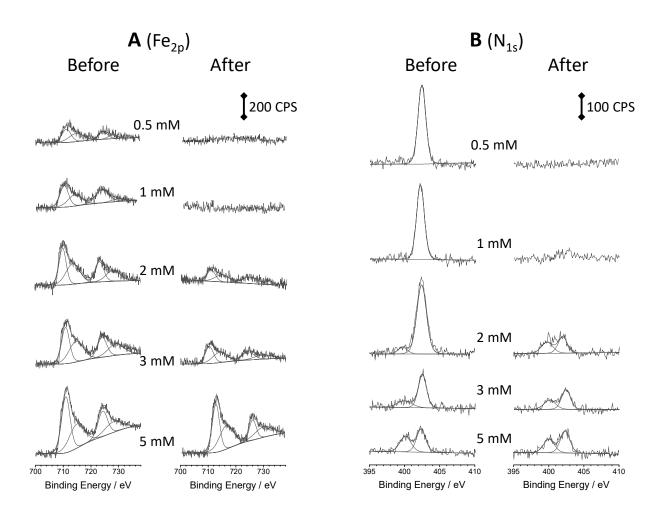
**Figure 4.** High-resolution XPS spectra for (A) iron (2p) and (B) nitrogen (1s) obtained using mesoporous silica films modified ITO electrodes prepared from a starting sol containing TEOS, CTAB, and various concentrations of  $Fe(Htrz)_3$  complex (from 0.5 to 5 mM), respectively before and after film treatment in 0.1 M HCl in ethanol.
