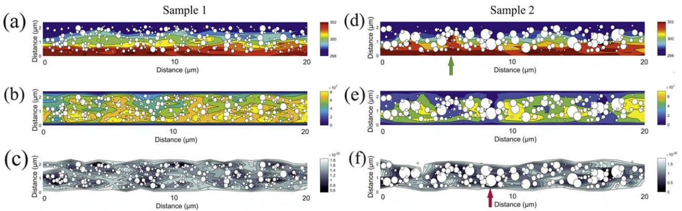
**Figure 4.** Simulated map of (a)/(d) temperature distribution, (b)/(e) heat flux and (c)/(f) volume distribution (white area present no porosity, while dark area are representative of high porosity) in Sample 1/Sample 2, assuming 55% of hole overlap. The white circles correspond to the overlapping pores present in the samples.
