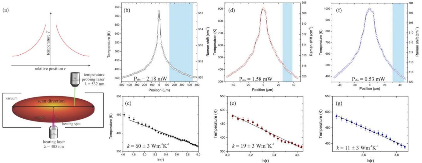
**Figure 2.** (a) Schematic of the two-laser Raman thermometry set-up and an example of a temperature profile of the sample. Temperature profiles and temperatures as a function of  $\ln(r)$  for: (b), (c) non-patterned, 100 nm thick membrane. (d), (e) Disordered porous membranes with filling fraction of 25%. (f), (g) Disordered porous membranes with filling fraction of 37%.
