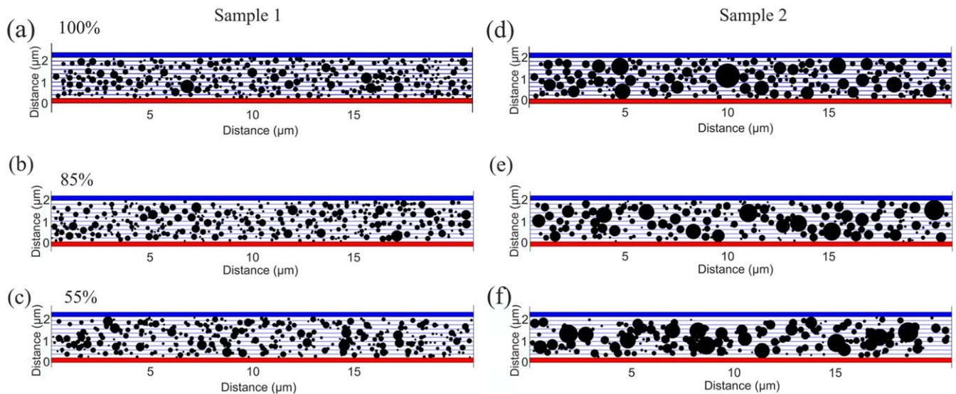
**Figure 3.** Pore distribution used in Monte Carlo simulations. Sample 1: (a) no overlap (100%), (b) 85% possible overlap (c) 55% possible overlap. Sample 2: (d) no overlap, (e) 85% possible overlap (f) 55% possible overlap. Red and blue rectangular represent the hot and the cold thermostats respectively.
