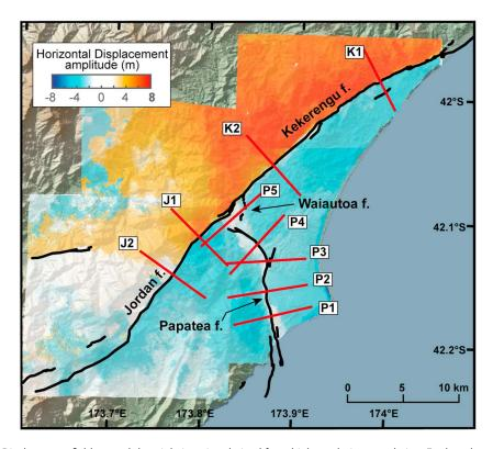
**Figure 2.** Displacement field around the triple junction derived from high-resolution correlation. Earthquake surface ruptures are indicated in black (Langridge et al., 2018). Color corresponds to the amplitude of horizontal displacement (positive towards north east). Low color saturation along the Papatea fault indicates off-fault damage. The red lines show the position of displacement profiles (see also Figure S1).
