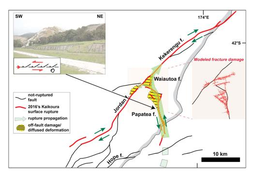
**Figure 4.** Summary of the preferred rupture path and associated fracture damage: Photo inset shows the observed surface damage on the Papatea fault (S42°08′47″, E173°52′01″). In addition to the main strike-slip scarp with some thrust, systematic westward branching with normal motion can be seen, which is best explained by left-lateral rupture propagating from the south. The yellow dashed areas correspond to the main areas of damage, from optical correlation and field observation.
