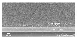
Fig. 3. SEM image (tilted at  $30^{\circ}$ ) of the monolayer of AgNPs deposited on thermally grown silica layer.
