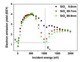
Fig. 2. EEY from very thin silica layers.
