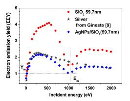
Fig. 4. Comparison of the EEY from SiO<sub>2</sub> ( $d_2 = 59.7$  nm), silver surface (adapted from [9]) and a structure of monolayer of AgNPs deposited on SiO<sub>2</sub> (59.7 nm) on Si-substrate.
