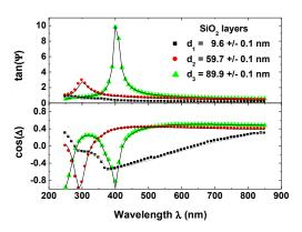
Fig. 1. Recorded ellipsometric spectra (dots) and the simulated spectra (lines) for the studied  $SiO_2$  layers.
