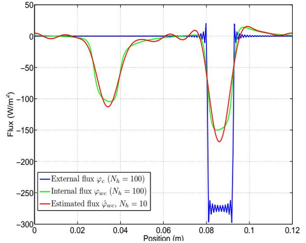
Figure 9: External cold flux ( $\varphi_c$ ) and internal cold wall fluxes ( $\varphi_{wc}$  and  $\hat{\varphi}_{wc}$ ).
