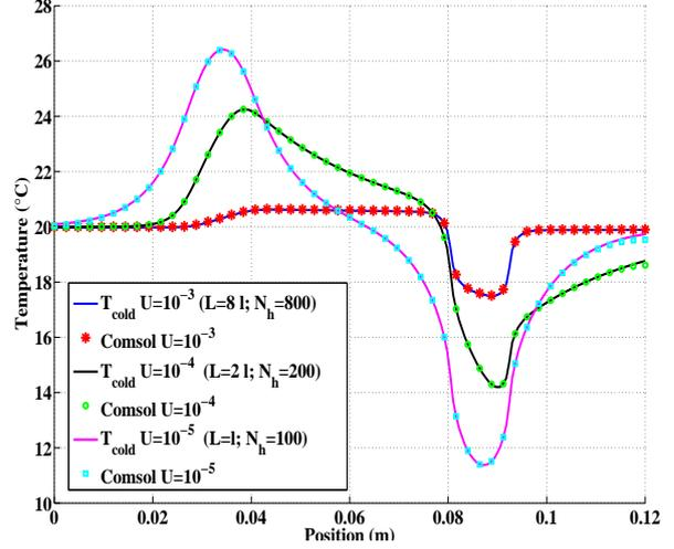
Figure 2: Comparison analytical/numerical temperature on hot face for different mean velocities  $U$  (in m/s).
