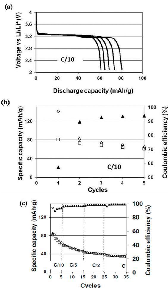
**Figure 5.** (a) Discharge capacity profiles at C/10, (b) charge (□) and discharge (◇) capacity and coulombic efficiency (▲) as function of cycles at C/10, (c) charge/discharge capacity as a function of the current rate.
