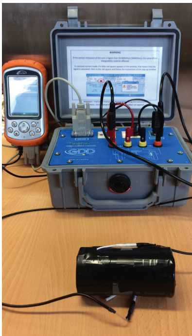
Figure 2. SCIP from GDD Inc. used for the time-domain measurements with four electrodes (A, B, M, and N). We used the following set of time-on: 1.0, 2.0, and 4.0 s, and we stack four times. We use 20 windows respecting a Cole-Cole distribution. We use an imposed voltage of 3 V.
