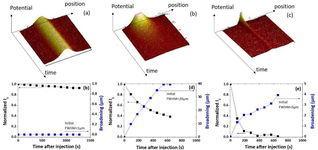
**Fig. 7.** Evolution of surface potential profile (a-c) and normalized  $I_s$  and broadening (d-e) as a function of time after injection for  $\text{SiO}_x\text{N}_y$  layers elaborated by plasma process with different gas ratio  $\gamma$  [76]: (a,d)  $\gamma=100$ , (b,e)  $\gamma=10$  and (c,f)  $\gamma=5$ . Charge injection in contact mode during 1min at 25V.
