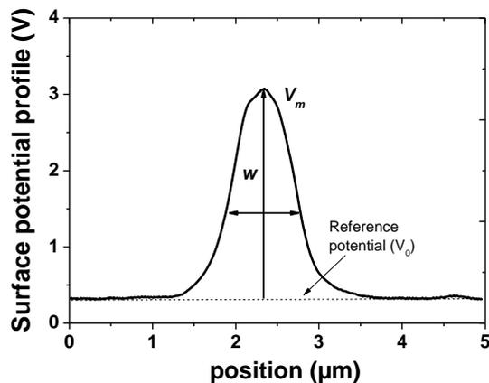
**Fig. 6.** Surface potential profile cross-section over contact point for punctual charge injection (2D surface potential map is depicted on Fig. 5.b).
