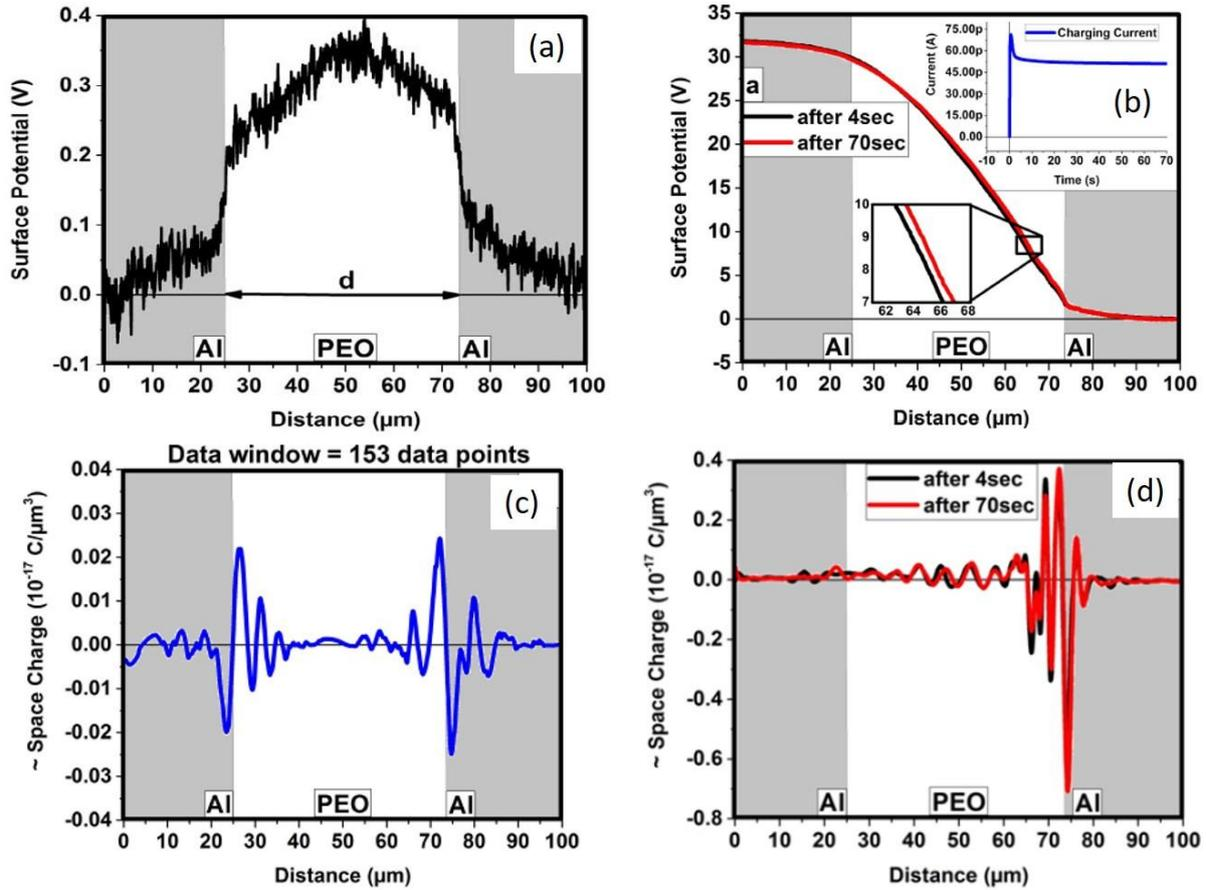
**Fig. 10.** Surface potential profile measured by KPFM over Al/PEO/Al structure (a) without applied bias and (b) 30V (ground) applied on left (right) electrode. Resulting space charge density profile obtained using SG-SDM method (c) without applied bias and (d) 30V (ground) applied on left (right) electrode. (Reproduced from Faliya et al [84])
