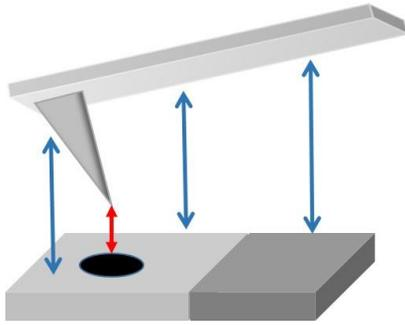
**Fig. 2.** Contribution of parasitic capacitance (blue arrow) compare to main contribution (red arrow) during KPFM measurement over a spot.
