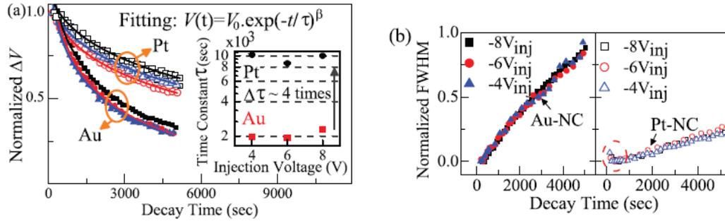
**Fig. 8.** Time dependence of normalized (a) maximum potential and (b) FWHM for sample with Au and Pt nanoparticles after charge injection of -4V, -6V and -8V during 10 s. The inset shows characteristic time constant extracted from the curve fitting (Reproduced from Lwin et al 2011).
