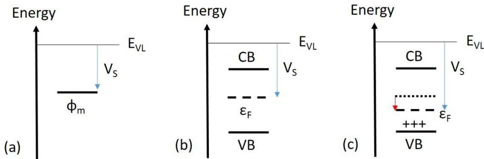
**Fig.1.** Energy level of (a) metal and (b) semiconductor or dielectric material with the corresponding surface potential  $V_S$ . (c) In presence of doping (semiconductor) or charges (dielectric) the surface potential is modified. Positive charges induce surface potential increase.  $\epsilon_F$  is the Fermi level. CB and VB are the conduction and valence bands, respectively.  $E_{VL}$  is the vacuum level.
