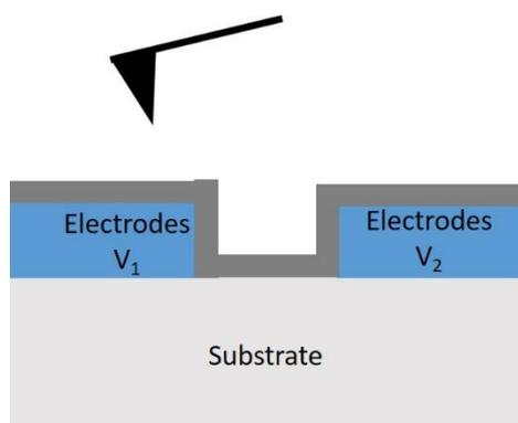
**Fig. 9.** KPFM configuration during measurement over real device under bias. In grey, dielectric or semiconductor active probed layer.
