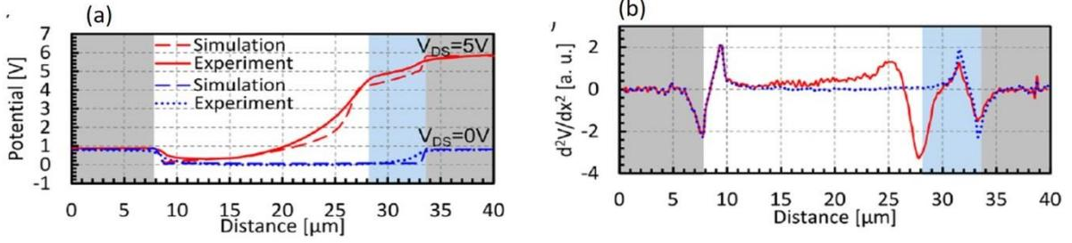
**Fig. 11.** (a) Comparison of surface potential profile measured by KPFM and simulated by TCAD software at  $V_{DS} = 0 V$  and  $V_{DS} = 5 V$  when  $V_{GS} = 0 V$ . (b) Calculated second derivative of the measured surface potential at  $V_{DS} = 0 V$  (dashed line) and  $V_{DS} = 5 V$  (solid line) represent the measured charge profiles (Reproduced with permission from Kryvchenko et al [90]. Copyright (2016) American Chemical Society)
