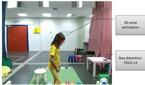
Fig. 4: The detected pose is shown along with the detected bounding box surrounding the robot’s head.
