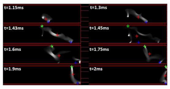
**Figure 7.** Views of the simulated net emission coefficient pictures treated with the arc position software showing with green, blue and red dots the positions of the upper arc root, lower arc root and global position of the arc for a peak current of 1608 A
