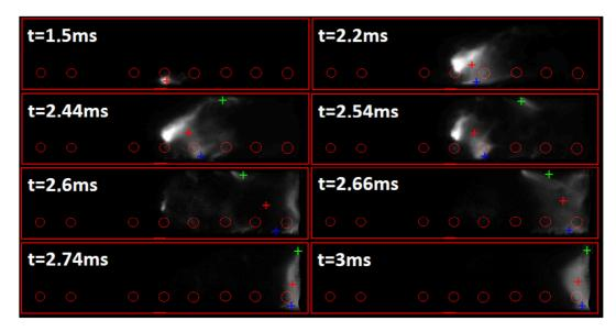
Figure 6. High-speed camera frames treated with the arc position software showing with green, blue and red dots the positions of the upper arc root, lower arc root and global position of the arc for a peak current of 1590 A
