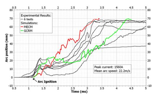
Figure 8. Experimental and simulated arc movements for fully open gas exhausts at medium current
