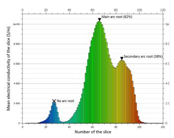
Figure 3. Example of arc root determination on one electrode
