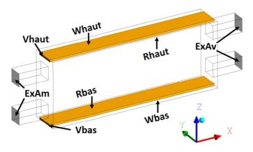
Figure 2. Simplified arc chamber geometry studied
