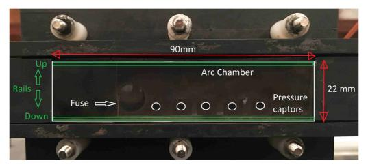
Figure 5. Rectangular geometry for experimental and model studies
