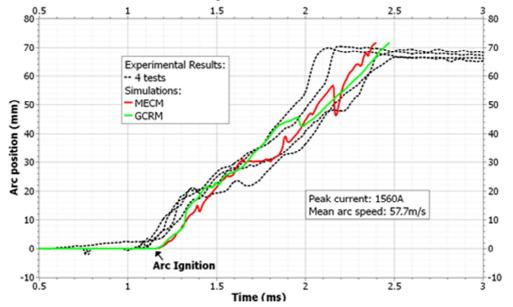
Figure 9. Experimental and simulated arc movements at medium current with closed upstream exhausts
