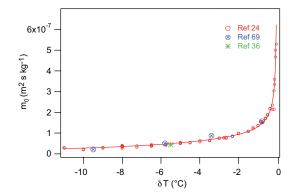
**Figure 15.** Mobility of elementary edge dislocations as a function of the temperature difference  $\delta T = T - T_{NA}$  (adapted from Ref. [30]). Errors on the mobility measurements are of the order of ±10%.
