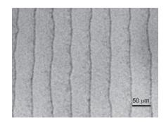
Figure 16. Geometrical elementary dislocations decorated by nanoparticles observed in transmission microscopy. The sample thickness is 20  $\mu$ m and the concentration of nanoparticles is 0.225 wt % (from Ref. [30]).
