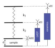
**Figure 12.** Equivalent mechanical model of the rheometer. The linear variable differential transformer (LVDT) is a very precise linear displacement transducer. It is used to measure a(t) when the cell is filled with the LC and u(t) when the cell is empty.
