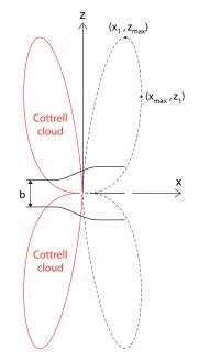
**Figure 4.** Cottrell cloud (red solid line) and anti-cloud (blue dashed line) around an edge dislocation in a smectic A LC (from Ref. [28]).
