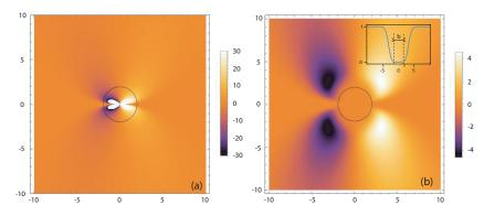
**Figure 5.** Density plot of the elastic potential. (a) raw potential. It strongly diverges inside the white regions; (b) smoothed potential  $\overline{W}(x,z) \equiv W(x,z)f_c(r)$ . The function  $f_c(r)$  is shown in the inset. The two circles represent the core of the dislocation. The lengths are given in units of  $\lambda$  and the potentials in units of  $k_BT$  (from Ref. [28], with kind permission of the European Physical Journal).
