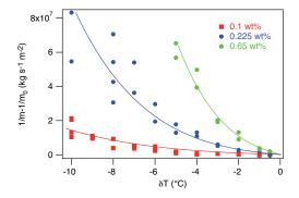
**Figure 17.** Shift between the reciprocal of the mobility and its value in pure 8CB as a function of temperature. The solid lines are the best fit with the model by taking  $\delta V \sim 27 \text{ nm}^3$  (adapted from Ref. [30]).
