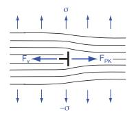
**Figure 3.** Peach and Koehler force and viscous force acting on an edge dislocation when the layers are dilated ( $\sigma > 0$ ).
