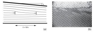
**Figure 11.** Geometrical dislocations (**a**) and their aspect under the microscope between crossed polarizers close to the SmA-SmC phase transition (**b**) (photo by S. Lagerwall, 1978).
