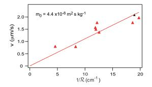
**Figure 10.** Dislocation velocity *v* measured in the asymptotic regime as a function of the curvature of the meniscus  $1/\mathcal{R}$  (Reprinted with permission from Phys. Rev. E, 62, 3747 (2000). Copyright 2000, American Physical Society).
