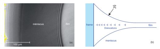
**Figure 9.** (a) typical appearance in reflecting microscopy of the meniscus formed between a film(on the right) and the frame (on the left). From the interference fringes observed in the thin region of the meniscus, the radius of curvature of the meniscus can be deduced; (b) model of meniscus of radius of curvature  $\mathcal{R}$  filled with dislocations (adapted from Ref. [9]).
