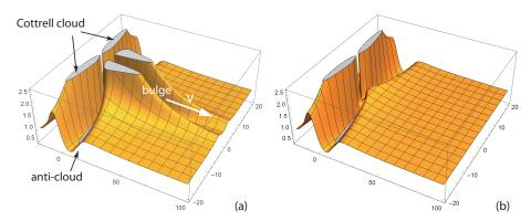
**Figure 6.** 3D plots of the dimensionless concentration field  $\bar{c}(x, z)$  numerically calculated with the FEM when  $D_{\perp} = 0$  (**a**) and  $D_{\perp} = D_{\parallel}$  (**b**). In this simulation, the layers are compressed and v = 0.1 mm/s. In these plots,  $1/e < \bar{c} < e$ ,  $-20 < \bar{x} < 100$  and  $-20 < \bar{z} < 20$  (adapted from Ref. [28], with kind permission of the European Physical Journal).
