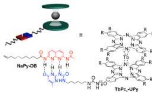
Fig 1. Sketch of the UPy-NaPy self-assembly mode used in this work for TbPc 2 anchoring on silicon surface (top left) and structures of the two components involved.
