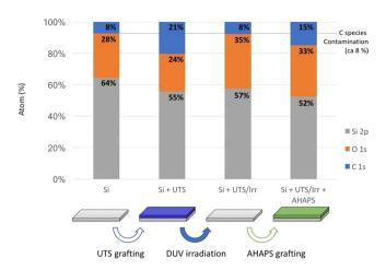
**Figure 5.** XPS analysis of the surface chemistry of a Si substrate showing the atomic composition of the surface of the Si substrate (i) before and (ii) after UTS grafting, (iii) after DUV irradiation (15 J/cm²) and iv) after regrafting of AHAPS on the irradiated substrate. The respective proportions of C, O and Si detected in the analyzed layer are given.
