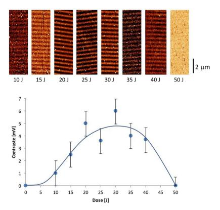
**Figure 7.** Evolution of the chemical contrast monitored by friction AFM (mV) on the patterns produced by interference irradiation of a UTS SAM (pattern width 300 nm). Top row: AFM images corresponding to each irradiation dose. Bottom: graph illustrating the contrast evolution. The blue line is a guideline for the eye.
