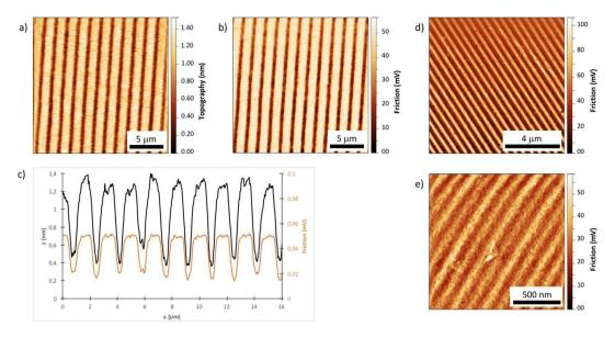
**Figure 6.** Typical images of chemical patterns obtained by DUV irradiation of an HTS SAM. (**a-c**) Topography, friction images and cross sections of the patterned surfaces (binary mask with 0.8 μm line width, 20 J/cm²). (**d,e**) Friction images of samples patterned by interference lithography with typical pattern widths of 300 nm and 75 nm, respectively, obtained for 30 J/cm².
