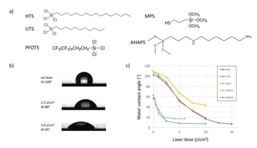
**Figure 2.** (a) Molecular structures of the silanes used in this study. (b) Images of water drops deposited on HTS surfaces before and after DUV irradiation at 2.5 and 5 J/cm<sup>2</sup>. (c) Modification of the water contact angle by DUV irradiation for HTS, UTS, MPS, PFOTS and AHAPS on Si substrates.
