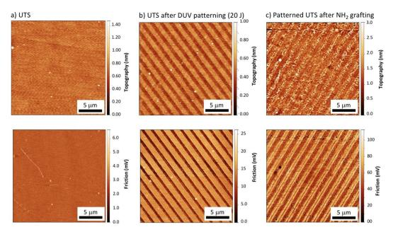
Figure 8. Contact mode AFM images, showing topography (top) and friction (bottom) images of (a) a UTS SAM surface, (b) UTS SAM surfaces patterned with DUV irradiation (20 J/cm²), with a 1.6 μm period chromium mask, and (c) the same patterned UTS surfaces after regrafting with an AHAPS precursor.
