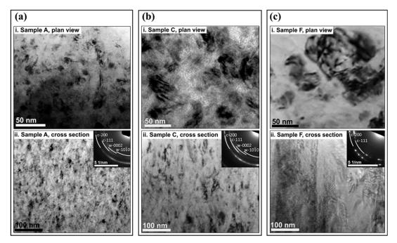
**Figure 8.** TEM micrographs of plan view (i), cross-section (ii) and selected area diffraction pattern (SAEDP) inset of as-deposited coatings A (a), C (b), and F (c), respectively. The SAEDPs of coatings A (a) and C (b) are indexed with mixed B1 and B4 phases, whereas the SAEDP of coating F (c) with a single phase B1 structure.
