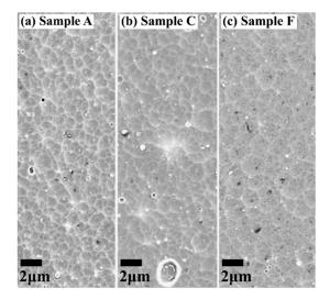
**Figure 10.** SEM micrographs showing the surface morphology of (**a**) coating A, (**b**) coating C, and (**c**) coating F.
