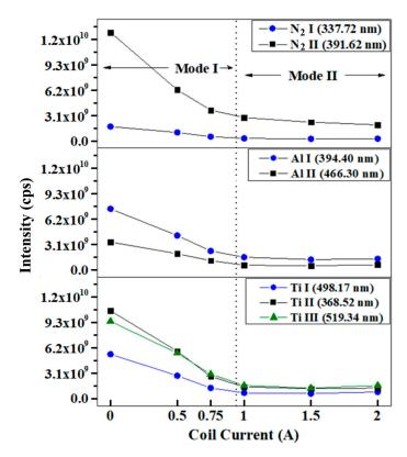
**Figure 6.** Intensities of detected optical emission lines of neutral Ti (498.17 nm), singly ionized Ti<sup>+</sup> (368.52 nm), doubly ionized Ti<sup>++</sup> (519.34 nm), neutral Al (394.40 nm), singly ionized Al<sup>+</sup> (466.30 nm), neutral N<sub>2</sub> (337.72 nm), and singly ionized N<sub>2</sub><sup>+</sup> (391.62 nm), as a function of coil current.
