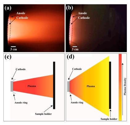
**Figure 3.** Side-view images (camera placed at  $87^{\circ}$  with respect to the surface normal) of the plasma plume emanating from the cathode are depicted for the cases of the 0 (**a**) and 2 A (**b**) coil currents. The pictures were acquired with an exposure of 4 ms. The cross-sections of the plasma plume are schematically drawn (not to scale) for the 0 (**c**) and 2 A (**d**) coil currents.
