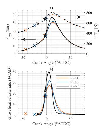
Figure 9. Pressure, temperature of the fresh gas mixture and gross heat release rate for various fuels at  $P_m = 1.0$  bar and  $\phi = 1.0$ . a) Solid lines: in-cylinder pressure, dotted lines: estimated fresh gas temperature. b) Solid lines: gross HRR. Crosses: SI timing, pentagrams: CA10.
