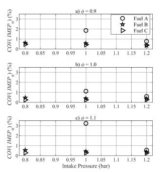
Figure 3. Coefficient of variation of the *IMEP*<sub>n</sub>
