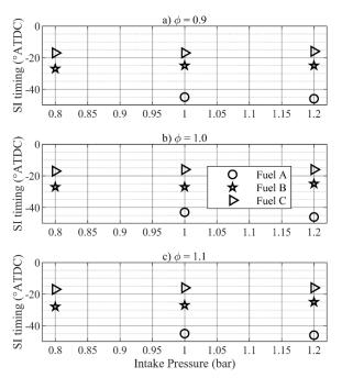
Figure 2. Spark Ignition timing at MBT under stable operating conditions.
