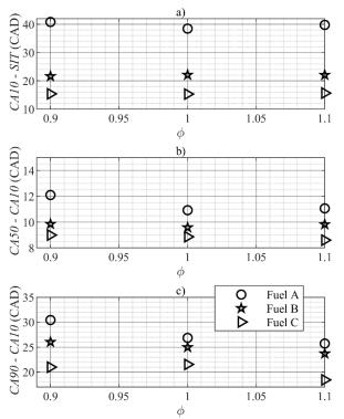
Figure 10. Combustion phases as functions of the equivalence ratio for  $P_{in} = 1.2$  har
