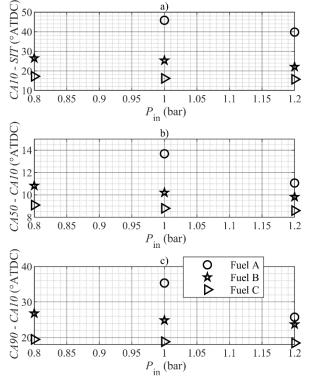
Figure 11. Combustion phases as functions of the intake pressure for  $\phi = 1.1$ .
