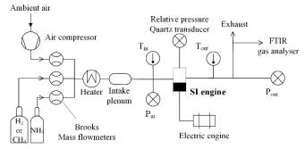
Figure 1. Layout of the experimental setup.
