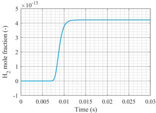
Figure 13. H<sub>2</sub> mole fraction in a homogeneous reactor with a stoichiometric NH<sub>3</sub>/air mixture under the conditions of Fig. 9a.
