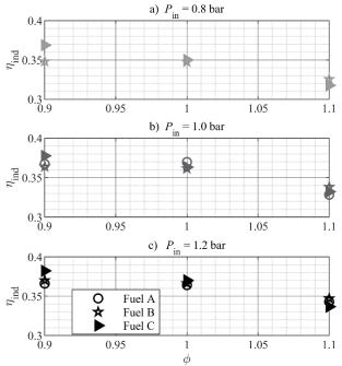
Figure 5. Indicated efficiency for the various fuels and intake pressures.
