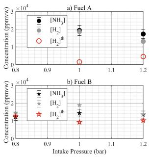
Figure 7. Comparison of NH<sub>3</sub> and H<sub>2</sub> exhaust concentrations for  $\phi = 1.1$ .
