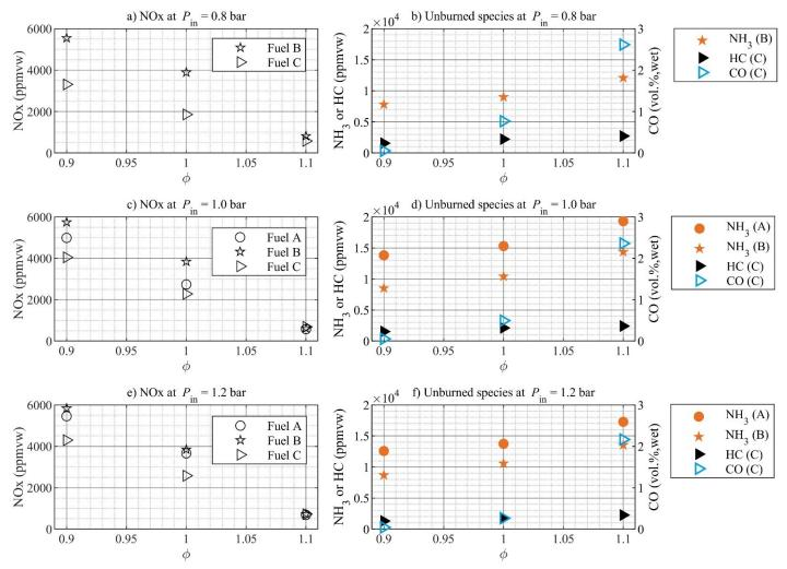
Figure 6. Pollutant concentrations in the wet engine exhaust. Left: NOx emissions. Right: Unburned species concentrations (NH $_3$  for ammonia-based fuels, HC and CO for methane fuel). Fuel A: 100% NH $_3$ , Fuel B: 85% NH $_3$  / 15% H $_2$ , Fuel C: 100% CH $_4$ .
