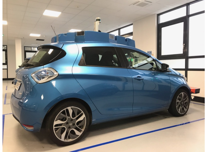
Fig. 2: The data acquisition platform ; the lidar stands on top of the vehicle
