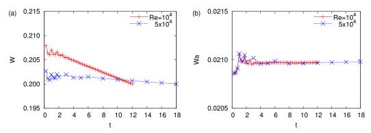
FIGURE 7. Time evolution of swirl parameter.  $Re = 10^4, 5 \times 10^4, W \approx 0.2$ . (a) W and (b) Wa.
