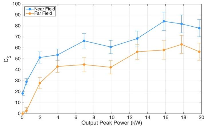
**Fig. 6.** Correlation between the experimental patterns at the GRIN-MMF output and the  $LP_{11}$  theoretical shape, upon the launched laser power, in the near-field (blue curve) and far-field (red curve), respectively.
