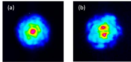
**Fig. 2.** Intensity patterns at the GRIN-MMF output recorded (a) for standard Kerr self-cleaning on a bell-shaped beam at 2 kW peak power, and (b) for Kerr self-cleaning on a  $LP_{11}$  profile, for specific beam coupling conditions and 4.5 kW peak power.
