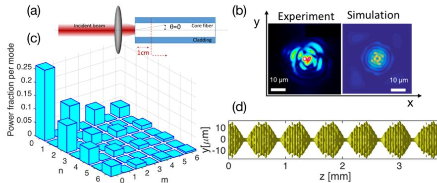
**Fig. 1.** (a) Experimental condition used for axial power coupling in the GRIN-MMF fiber, (b) Corresponding experimental and numerical near field intensity patterns after 1 cm of propagation in the GRIN-MMF, (c) Fraction of power coupled into the guided modes (Hermite-Gauss basis); (d) Iso-intensity surface (at 50% of the local maximum) upon the propagation distance  $z$ .
