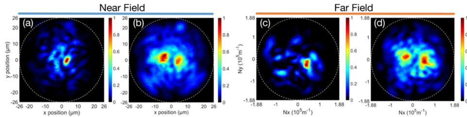
**Fig. 5.** Near field (a),(b) and far field (c),(d) intensity patterns at the GRIN-MMF output recorded in linear propagation regime (a, c) and in the nonlinear self-cleaning regime (b, d) for appropriate settings of the input coupling, in order to get self-cleaning of a  $LP_{11}$  mode. The white line corresponds to the core boundary in the near field images and to the NA in the far field images.
