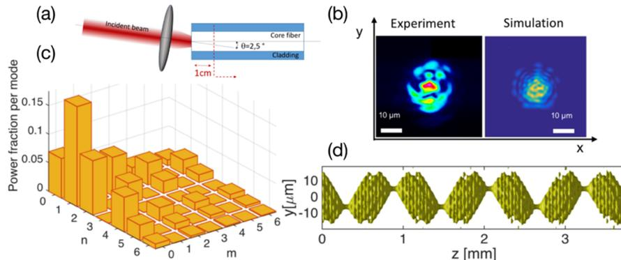
**Fig. 3.** (a) Experimental condition used for power coupling in the GRIN-MMF fiber with an input incidence angle of  $2.5^\circ$ ; (b) Corresponding experimental and numerical near field intensity patterns after 1 cm of propagation in the GRIN-MMF, (c) Fraction of power coupled into the guided modes (Hermite-Gauss basis), (d) Iso-intensity surface at 50% of the local maximum along the propagation distance  $z$ .
