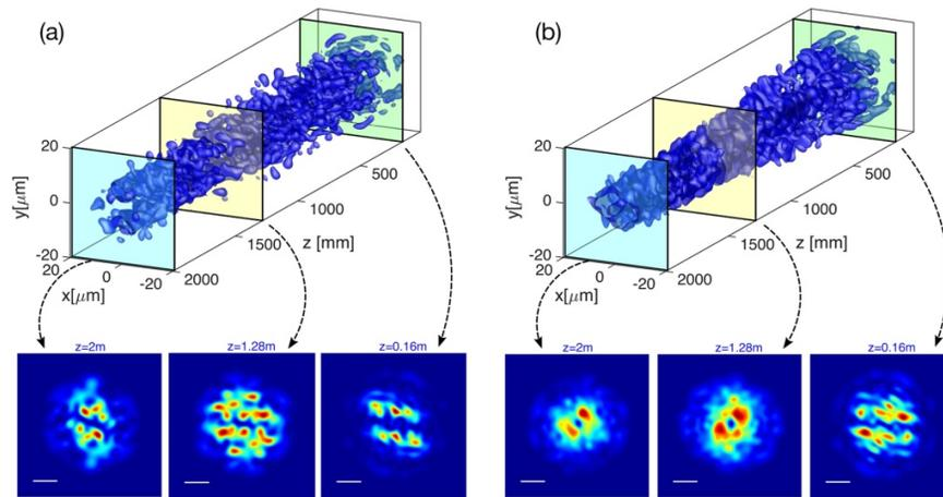
**Fig. 7.** Time-averaged numerical results (Iso-intensity surfaces at 50% of the local maximum) of beam propagation in a GRIN MMF. (a) absence of Kerr effect. (b) Kerr effect enabled. The insets show the beam intensities at three different positions along the propagation. White segment:  $10\ \mu\text{m}$ .
