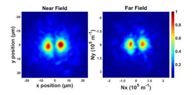
Fig. 4. Kerr beam self-cleaning on LP11 mode after adaptive shaping of the excitation beam wavefront (Peak power 34.5 kW). The occurrence of similar patterns in the near and far fields demonstrate the major content of the LP11 in the output modal population.
