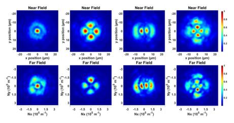
Fig. 5. Near field (top row) and far field (bottom row) images recorded after optimization of the input wavefront, in order to obtain a desired mode profile at the MMF output facet ( $LP_{02}$ ,  $LP_{21}$ ,  $LP_{12}$  and  $LP_{22}$  from left to right, respectively) at relatively high peak powers (31 kW, 31 kW, 29 kW and 29 kW, respectively).
