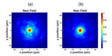
Fig. 2. (a) Standard Kerr beam self-cleaning obtained with a flat wavefront input beam and observed at the fiber output with a Peak power of 45 kW. (b) Kerr beam self-cleaning on the fundamental mode of the fiber after adaptive input wavefront shaping (Peak power 40 kW).
