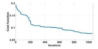
Fig. 3. Evolution of the cost function according to the iterations of the optimization process for Kerr self-cleaning on the fundamental mode of the GRIN MMF.
