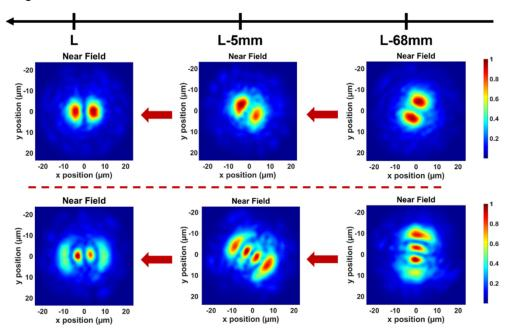
Fig. 9. Near-field images after optimized Kerr self-cleaning of two examples of LOMs (LP<sub>11</sub> top row, LP<sub>12</sub> bottom row) recorded at the fiber output (left column), then after cut back of the fiber by 5 mm whilst keeping the whole input conditions (center column), and after cut back by 68 mm (right column). Translational invariance of the cleaned beam was observed. Rotation of the patterns in the camera frame from left to right are due to fiber twist.
