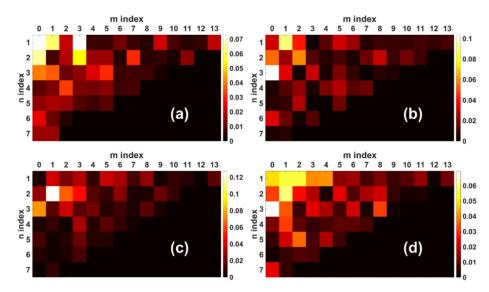
Fig. 6. Mode power distribution of the launched fields, in order to obtain self-cleaning on the  $LP_{01}$  (a),  $LP_{11}$  (b),  $LP_{12}$  (c), and  $LP_{21}$  (d) modes, respectively. Charts were computed from projections of the optimized wavefront profiles on the fiber mode basis. Color bars indicate the percentage of input mode power.
