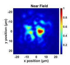
Fig. 7. Near field observed at a relatively low power (150 W), while keeping the input wavefront optimized for self-cleaning on a  $LP_{11}$  intensity pattern at high powers (e.g., see Fig. 4 above for reference).
