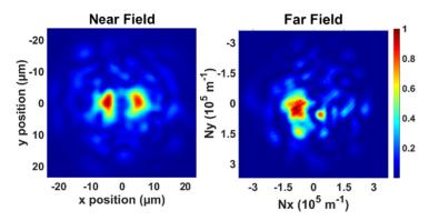
Fig. 8. Near field and far field images recorded after optimization of the input wavefront to get a  $LP_{11}$  intensity pattern at the MMF output in linear propagation regime. Although the figure on the left resembles a  $LP_{11}$  (with a strong background) the far field indicates  $LP_{11}$  is not the major modal contribution to the output field (left).
