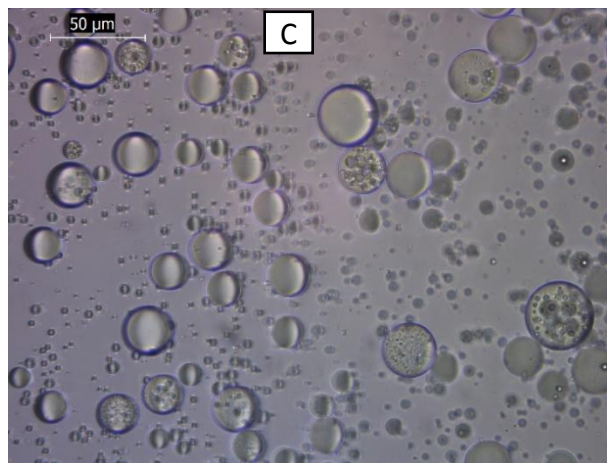
Figure 2: Microscopic images of the double emulsion prepared with \phi_{\mu} 40 %, \phi_M = 1 %, and \omega_R = 400 rpm: A) day 0 so right after preparation, B) day 6 and C) day 20.
