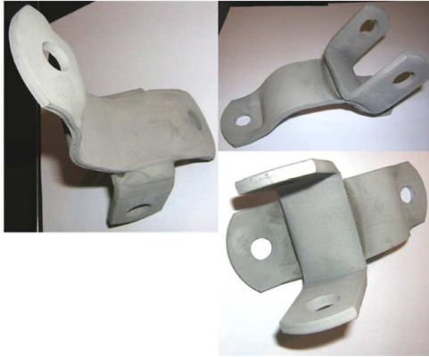
Figure 4. Complex-shape articles epanized at 400°C during 90 min (coating thickness = 25 μm).
