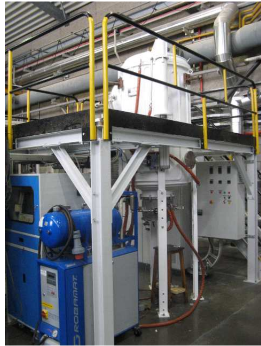
Figure 2. The equipment built to develop the process at a larger scale (Umicore). a) The vacuum vessel. b) An overall view of a development set-up.
