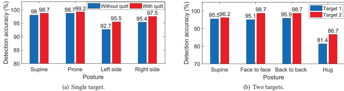
Fig. 28. Impact of target sleep posture. It can be seen that LungTrack operates well in all of the above scenes except when targets are hugging each other.
