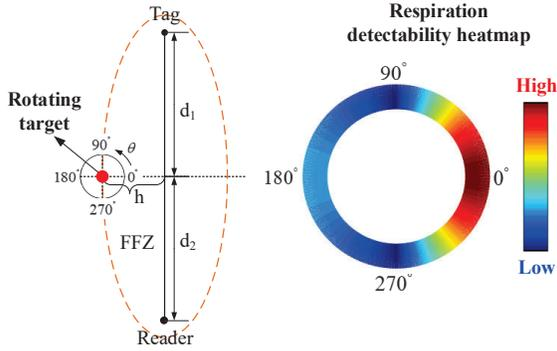
Fig. 7. Impact of target orientation  $\theta$  ( $k_{front} = 1$ ). Left: setup. Right: the visualization of respiration detectability. The red color indicates good detection performance, while the blue color indicates the performance is poor.
