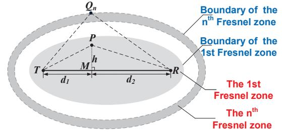
Fig. 2. An illustration of the Fresnel zones.  $T$  and  $R$  represent the signal transmitter and receiver, respectively.  $P$  represents a human target when it is located in the first Fresnel zone, and  $Q_n$  represents a human target in the  $n^{\text{th}}$  Fresnel zone.
