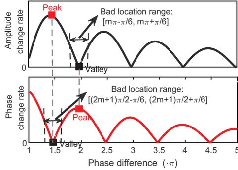
Fig. 9. Complementary principle between amplitude and phase information for respiration sensing (in  $2^{\text{nd}} - 5^{\text{th}}$  Fresnel zones,  $m = 1, 2, \dots, 5$ ). The greater rate of signal amplitude/phase change indicates the better respiration sensing capability.
