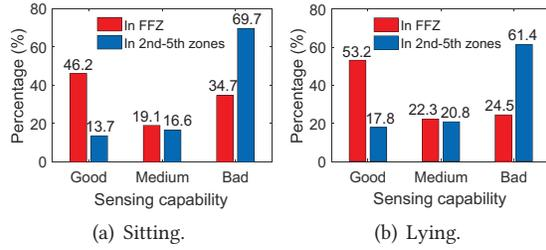
Fig. 19. Respiration detectability at two postures. The better sensing capability for lying posture is because when target lies, the respiration causes movement at both front chest and back while when target sits, the respiration causes larger front chest displacement.
