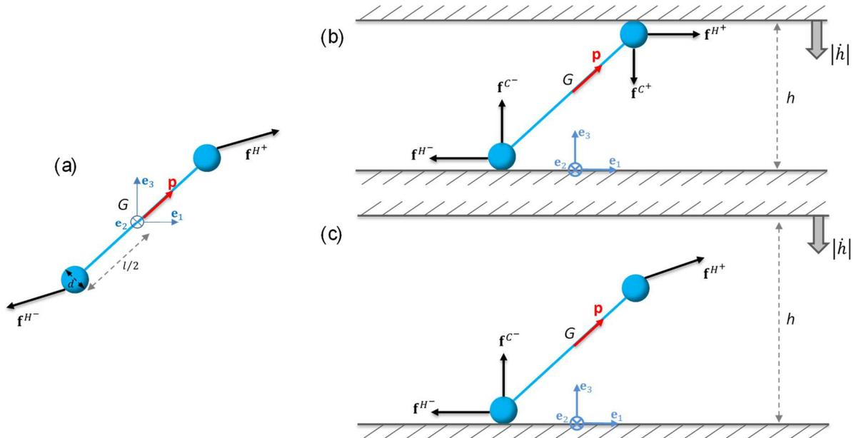
Figure 3. Fiber  $i$  modeled by a dumbbell. (a) Unconfined lubricated squeeze flow with hydrodynamic forces  $\mathbf{f}_i^{h^\pm}$  exerted on the upper and lower beads. (b) Confined lubricated squeeze flow with centred dumbbell, hydrodynamic  $\mathbf{f}_i^{h^\pm}$  and contact  $\mathbf{f}_i^{c^\pm}$  forces exerted on the upper and lower beads. (c) Confined lubricated squeeze flow with only one contact with the lower wall.
