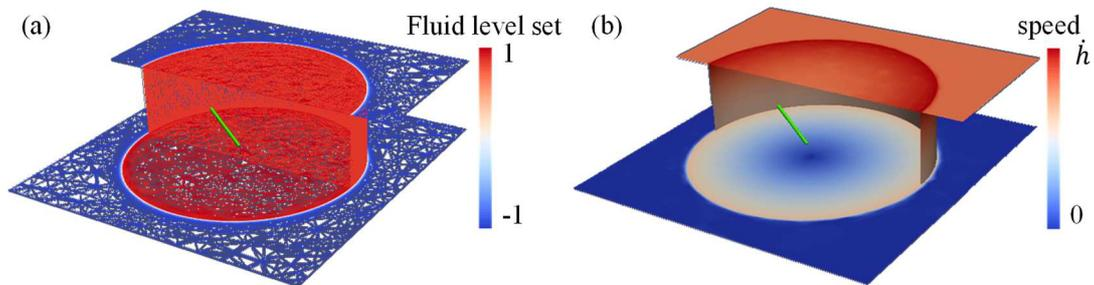
Figure 2. (a) Iso-values of the truncated fluid level-set  $\varphi_f$  and adaptive mesh used to run the simulation, displayed on platens and fluid domains. (b) Iso-values of the velocity magnitude shown on platens and fluid domains.
