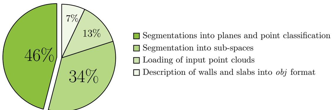
(b) Processing of the main block of the office building (1000 m<sup>2</sup>, ~ 16M points) – Time required: 19 min
