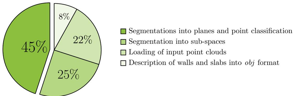
(a) Processing of the individual house (200 m<sup>2</sup>, ~ 10M points) – Time required: 8 min
