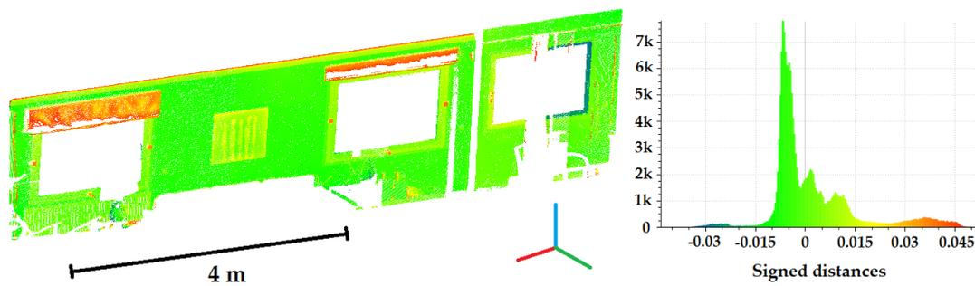
(a) Point cloud of an indoor portion of a façade wall
