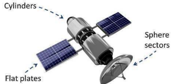
Figure 2: Examples of simple shapes composing a satellite 5
