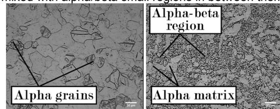
Fig. 1. Microstructure of pure titanium and Ti-6Al-4V.
