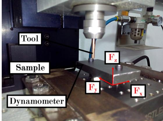
Fig. 3. Cutting force measurement directions.
