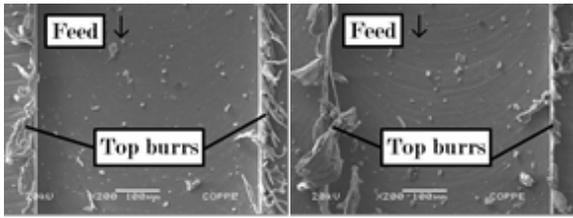
Fig. 9. Scanning electron microscope images: a) CP-Ti – 1.0 μm/th; b) CP-Ti – 3.5 μm/th; c) Ti-6Al-4V – 1.0 μm/th; d) Ti-6Al-4V – 3.5 μm/th.
