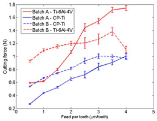
Fig. 6. Experimental cutting force results.
