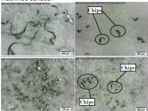
Fig. 10. Digital microscope images of chips: a) CP-Ti – 0.5 μm/tooth; b) CP-Ti – 4.0 μm/tooth; c) Ti-6Al-4V – 0.5 μm/tooth; d) Ti-6Al-4V – 4.0 μm/tooth.
