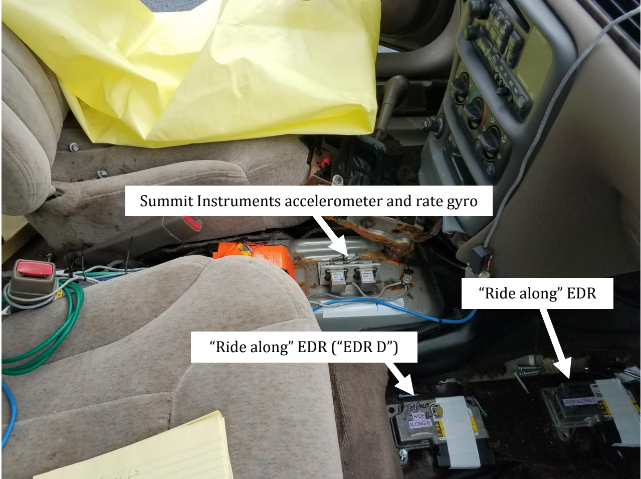
Figure 7: Photograph showing accelerometer and two "ride along" ACMs inside Chevy Malibu cabin.
