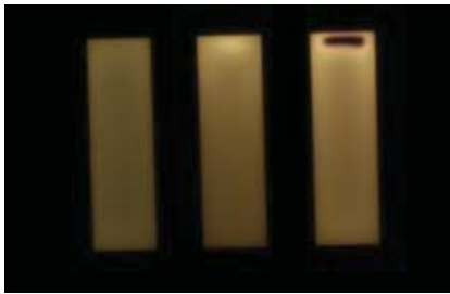
Fig. 2. Photos of a degraded OLED under a strong current (appearance of black spots)
