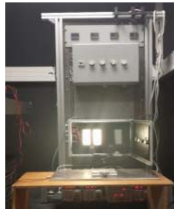
Fig. 5. Experimental bench of OLED aging tests
