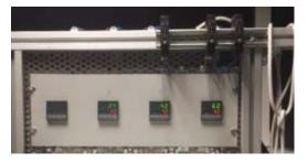
Fig. 4. Temperature controllers and meters (in hours)
