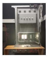
Fig. 5. Experimental bench of OLED aging tests
