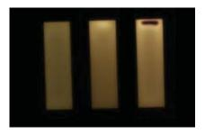
Fig. 2. Photos of a degraded OLED under a strong current (appearance of black spots)
