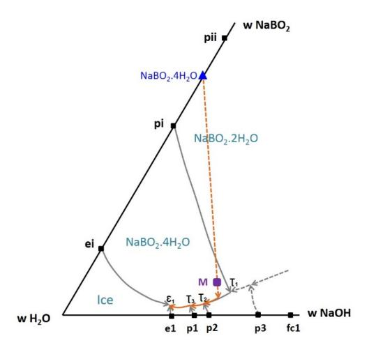
$\begin{array}{l} \textbf{Figure 9.} \ Close-up \ of polythermal \ diagram \ of the ternary \ system \ NaBO_2-NaOH-H_2O \ presented \ in \ Figure 8, \ mixture \ point \ M \ (24.8 \ w\% \ NaOH \ and 5.16 \ w\% \ NaBO_2) \ sample \ located \ on \ solid-phase \ domain \ of \ NaBO_2.4H_2O \ and \ in \ the \ triangle \ of \ solid-phases \ NaBO_2.4H_2O-NaOH.7H_2O-NaOH.7H_2O-NaOH.5H_2O. \end{array}$
