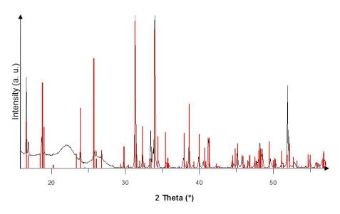
Figure 8. Powder X-Ray pattern of solid phase of the crystallization domain of metaborate superior hydrate: NaBO<sub>2</sub>.4H<sub>2</sub>O, ICDD file n° 04-011-5978 represented in red (mixture point composition: 15 w% NaBH<sub>4</sub>; 10 w% NaOH and 75 w% H<sub>2</sub>O).
