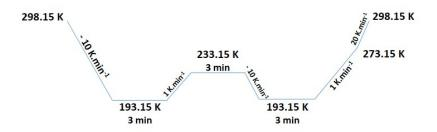
Figure 2. Temperature scanning profile adopted for DSC analyses.
