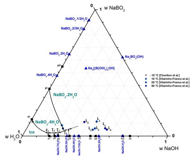
Figure 7. Polythermal diagram of the ternary system  $NaBO_2$ -NaOH- $H_2O$  with binary invariant temperatures ( $\blacksquare$ ), different hydrates ( $\blacktriangle$ ). Definition of different domains of crystallization with the isobaric invariants points. Proposition of monovariant lines: isotherm at -10 °C by Churikov et al. [12] and isothermal at 10, 25 and 50 °C from previous experimental work [11].
