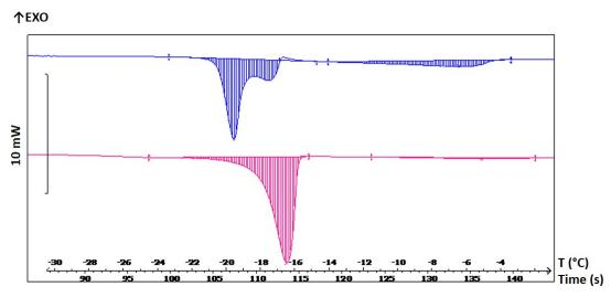
Figure 1. DSC thermogram of an aqueous ternary mixture M (24.8 w% NaOH - 5.16 w% NaBO<sub>2</sub>-70.04w% H<sub>2</sub>O) first results underscoring no repeatability on the phase transformation phenomena.
