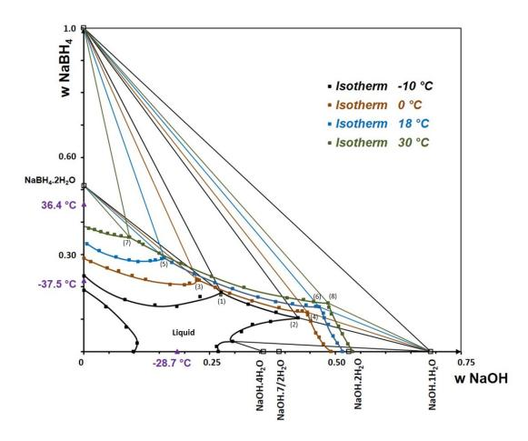
Figure 3. Superposition of the isotherms at -10, 0, 18 and 30 °C of the ternary system NaBH<sub>4</sub>–H<sub>2</sub>O–NaOH. Literature data from Churikov et al. [12] and Mikheeva and Breitsis [14].
