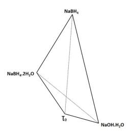
Figure 5b. Representation of the convex quadrilateral involving T<sub>0</sub>, transitory peritectic transformation.
