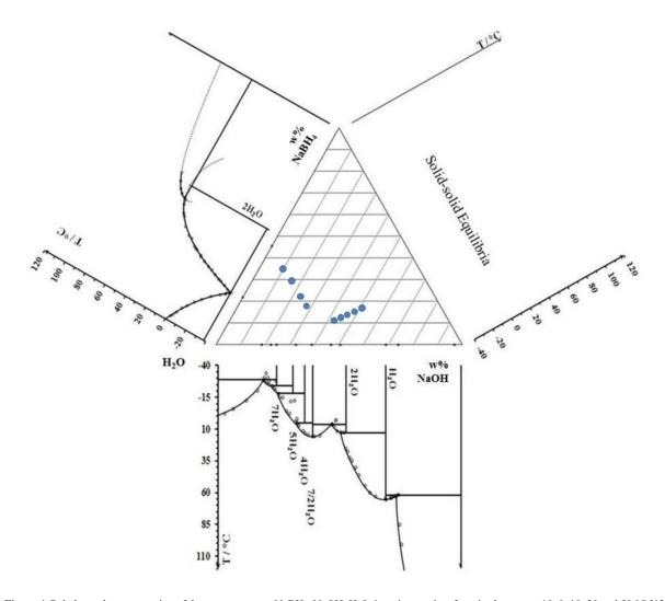
Figure 4. Polythermal representation of the ternary system NaBH<sub>4</sub>–NaOH–H<sub>2</sub>O, invariants points from isotherms at -10, 0, 18, 30 and 50 °C [12, 14] with the aqueous boundary binary systems on the edge: NaOH–H<sub>2</sub>O [19] and NaBH<sub>4</sub>–H<sub>2</sub>O [14, 18].
