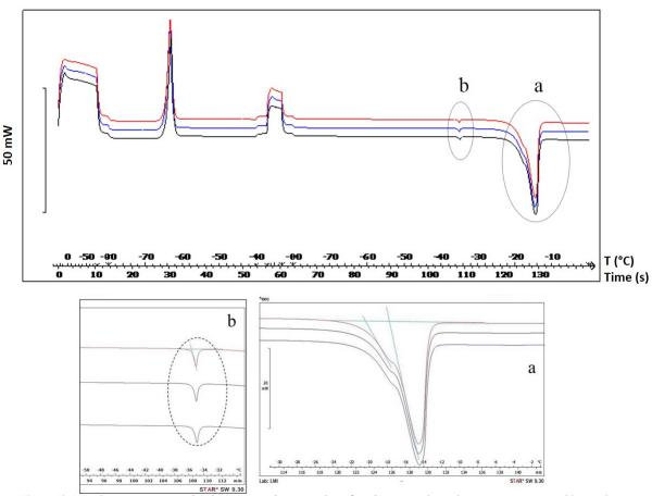
Figure 10. DSC thermograms presenting three consecutive run analyses for mixture sample M, the temperature range: -80 °C to 25 °C.
