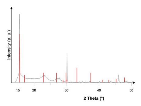
Figure 6. Powder X-Ray pattern of solid phase of the crystallization domain of borohydride superior hydrate: NaBH<sub>4</sub>.2H<sub>2</sub>O, ICDD file n° 00-036-1233 represented in red (mixture point composition: 25 w% NaBH<sub>4</sub>; 10 w% NaOH and 65 w% H<sub>2</sub>O).
