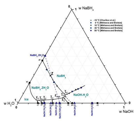
Figure 5a. Polythermal diagram of the ternary system NaBH₄-NaOH-H₂O with isobaric binary invariant transformations (■), different hydrates (▲). Definition of different domains of crystallization with the isobaric invariants points. Proposition of monovariant lines based on literature data: isotherm at −10 °C by Churikov et al. [12] and isotherms at 0, 18, 30 and 50 °C by Mikheeva and Breitsis [14].
