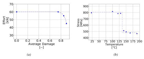
Fig. 1. Effect of damage on tensile strength: a); b) Tensile failure stress vs. temperature on a GFRP 1055/ES18 [2]
