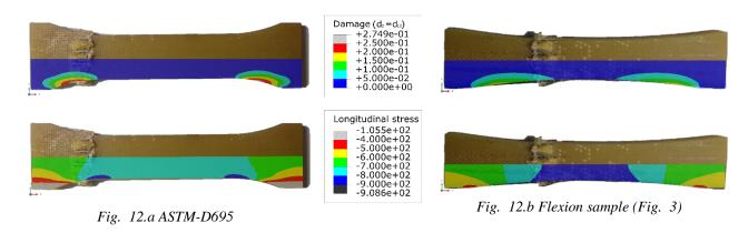
Fig. 12. ASTM-D695 samples vs FEM simulation
