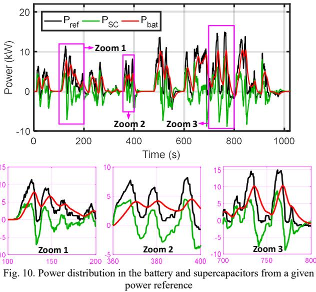
Fig. 10. Power distribution in the battery and supercapacitors from a given power reference
