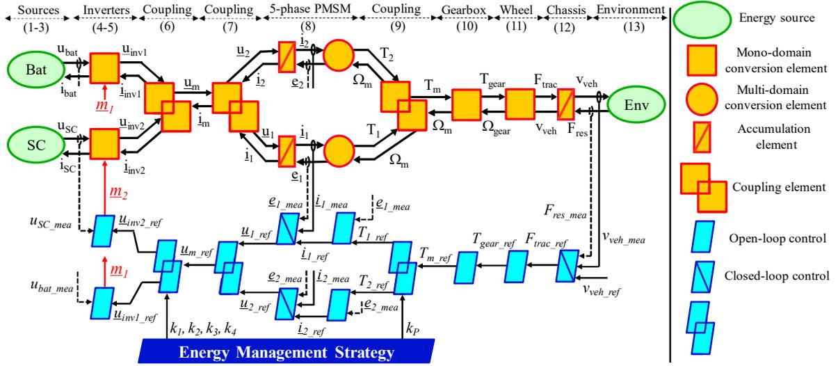
Fig. 2. Energetic macroscopic representation and inversion-based control of the studied electric vehicle
