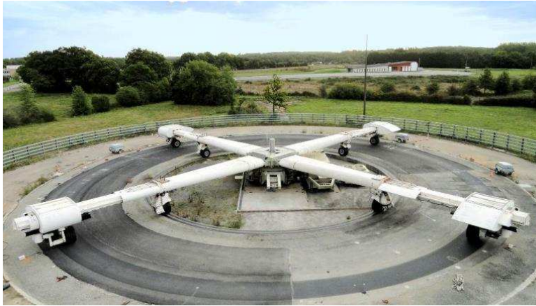
Figure 2. The IFSTTAR accelerated pavement testing facility
